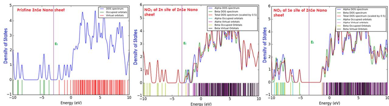
Fig. 4: DOS spectra of pristine and NO<sub>2</sub> adsorbed ZnSe Nano tube
