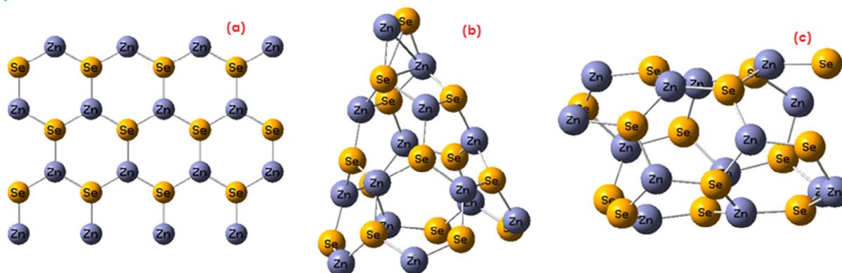
**Fig. 1: Pristine ZnSe nano sheet, nano cone and nano tube structures**
