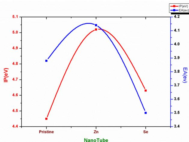
Fig. 5(c): IP and EA curves of pristine, NO<sub>2</sub> adsorption of Zn and Se sites of ZnSe nanotube
