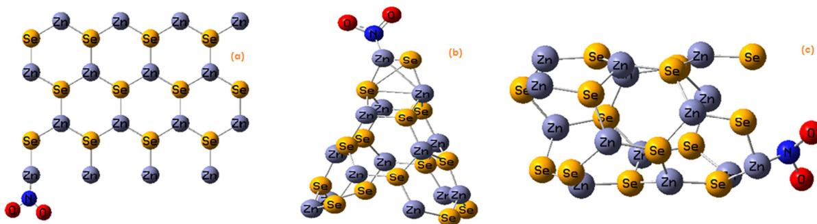
Fig. 6: NO<sub>2</sub> adsorption on Zn sites of ZnSe nanosheet, nano cone and nano tube structures
