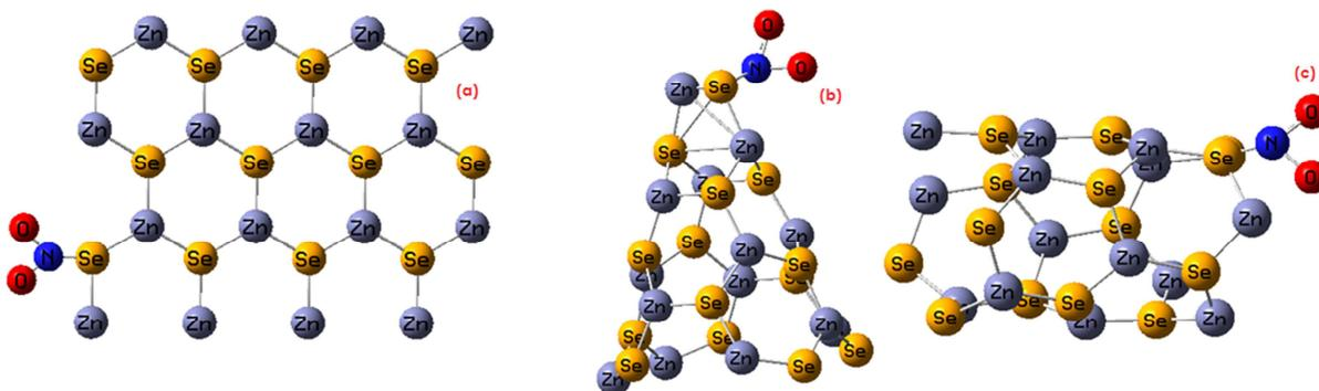
Fig. 7: NO<sub>2</sub> adsorption on Se sites of ZnSe nanosheet, nano cone and nano tube structuresTable 3 Adsorption energies of NO<sub>2</sub> at Zn and Se sites on the ZnSe nano structures
