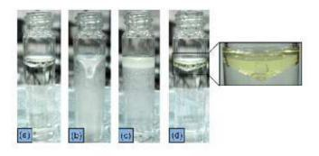
Figure 1. Illustration of the microextraction apparatus for directly suspended droplet LLLME: (a) addition of the organic solvent to the aqueous sample solution, magnetic stirrer is off; (b) the mixture is being agitated, extraction procedure; (c) separation of the tiny drop of the organic solvent and aqueous sample solution and then addition of the acceptor phase into the organic solvent, magnetic stirrer is off; (d) back-extraction procedure, magnetic stirrer is on [16]
