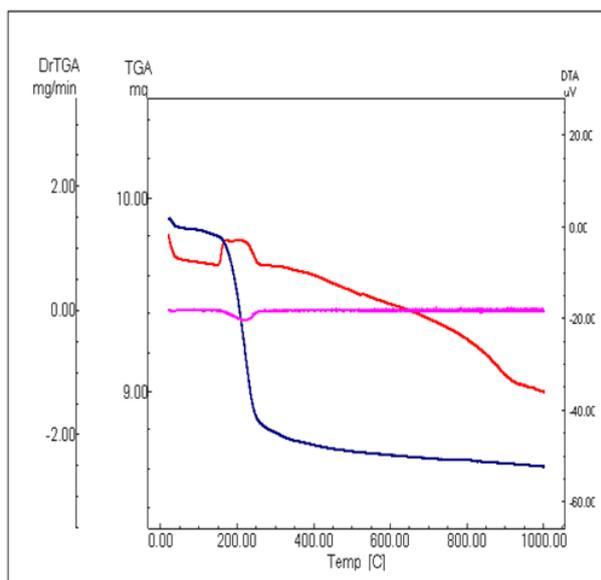
Figure 4: The profile of DTA and TGA curves of liquid crystal I<sub>1</sub>
