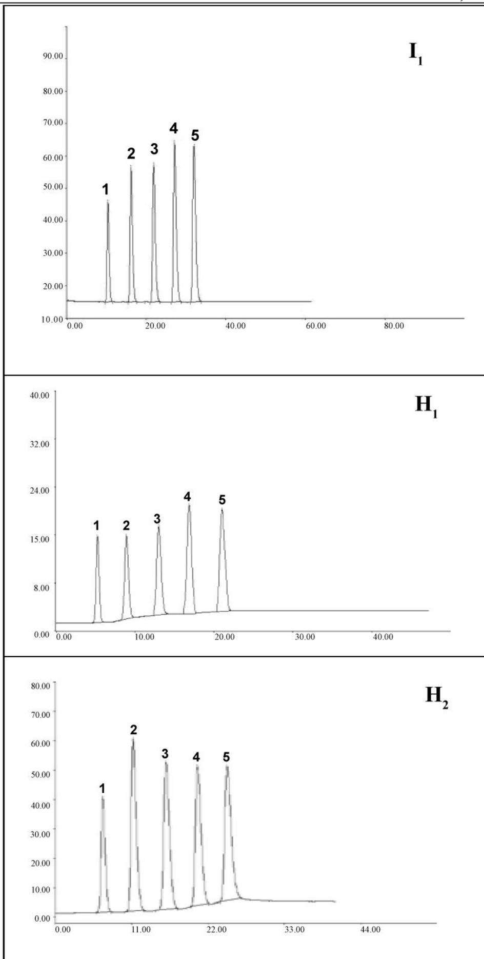
Figure 9: GC separation of paraffinic hydrocarbons (from 1-n-C<sub>6</sub>, to 5-n-C<sub>10</sub>) at optimum condition (80°C for 2 min; 20°C/min to 200°C; final time 10 min, 30 ml. min<sup>-1</sup>)
