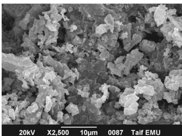
Figure 7: SEM images of liquid crystal H<sub>2</sub> as stationary phase
