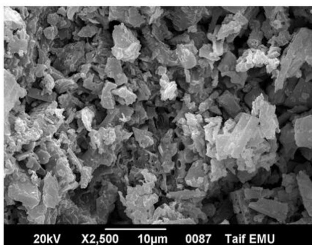
Figure 8: SEM images of liquid crystal I<sub>1</sub> as stationary phase
