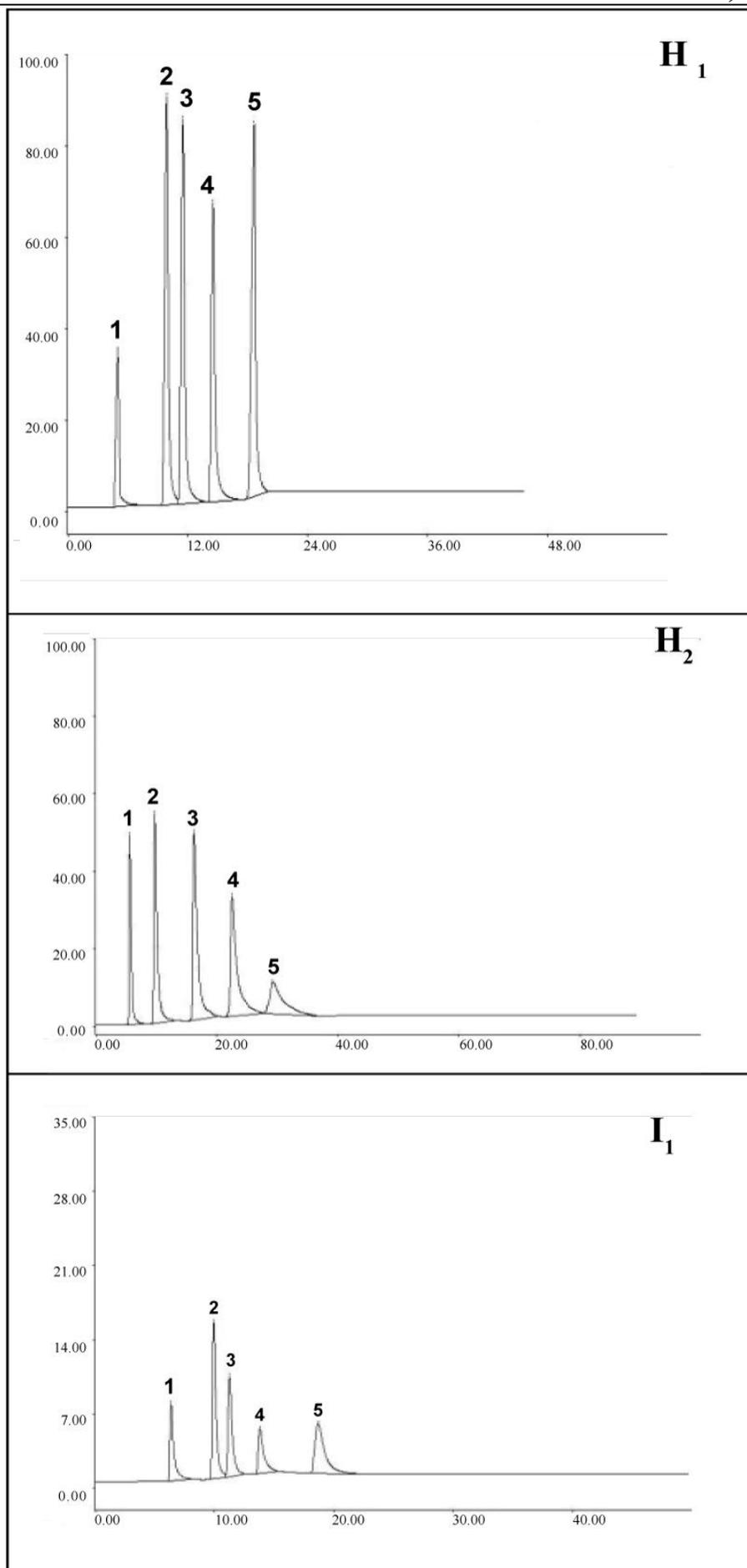
Figure 11: GC separation of Alcohols (from C<sub>2</sub>H<sub>5</sub>OH to C<sub>6</sub>H<sub>13</sub>OH), at optimum condition (80°C for 2 min; 20°C/min to 200°C; final time 10 min, 30 ml. min<sup>-1</sup>)
