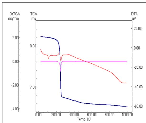
Figure 2: The profile of DTA and TGA curves of liquid crystal H<sub>1</sub>
