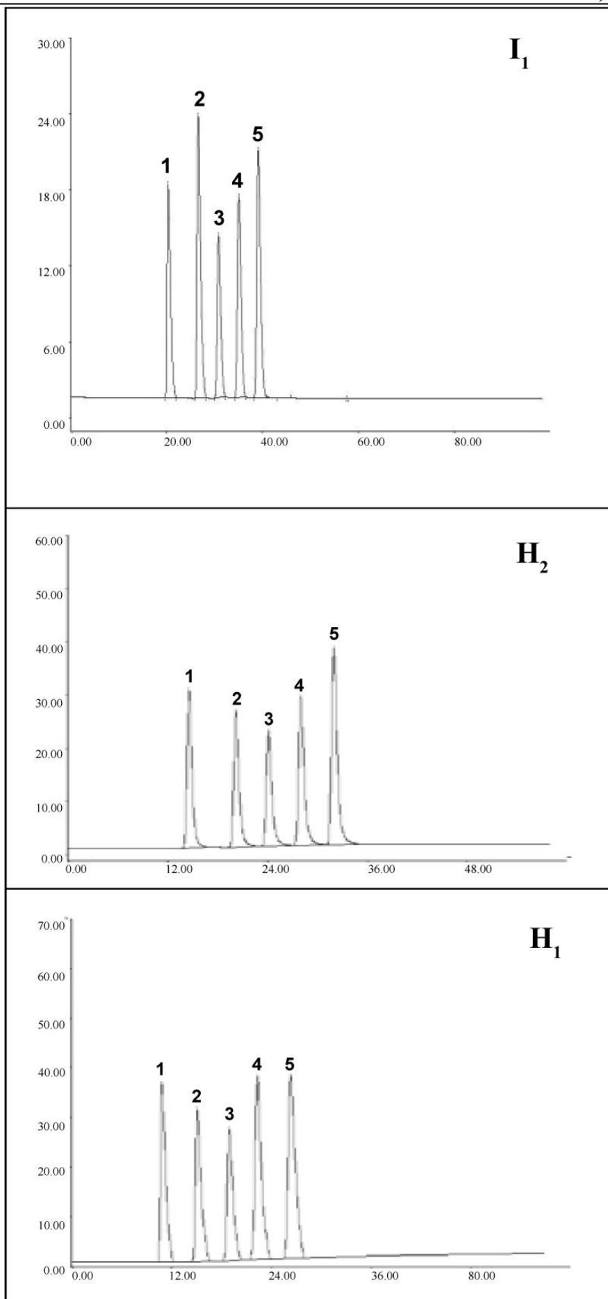
Figure 10: GC separation of (Benzene, toluene, ethylbenzene, propylbenzene and butylbenzene), at optimum condition (80°C for 2 min; 20°C/min to 200°C; final time 10 min, 30 ml. min<sup>-1</sup>)
