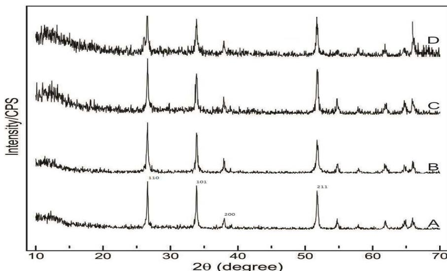
Figure 1. XRD Pattern of pure (A) and Al doped  $\text{SnO}_2$  (B, C and D)
