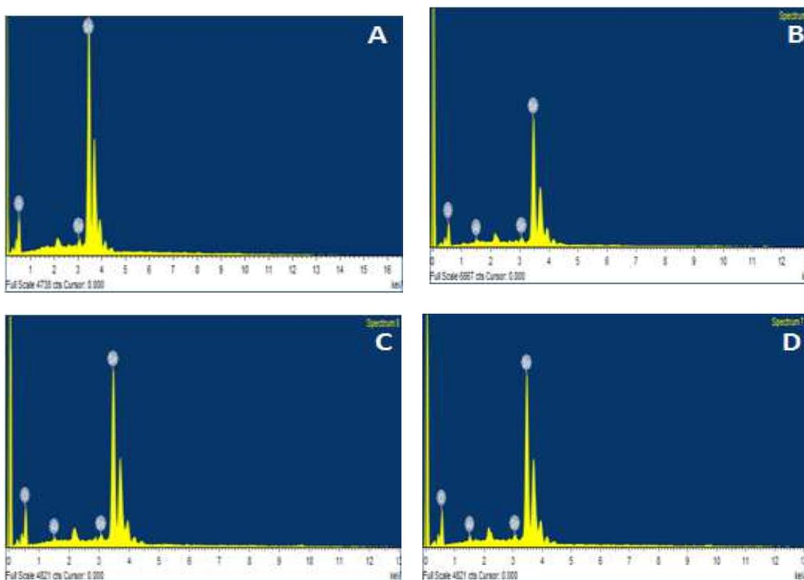
Figure 4. EDAX Spectrum of pure (A) and Al doped SnO<sub>2</sub> (B,C,D)
