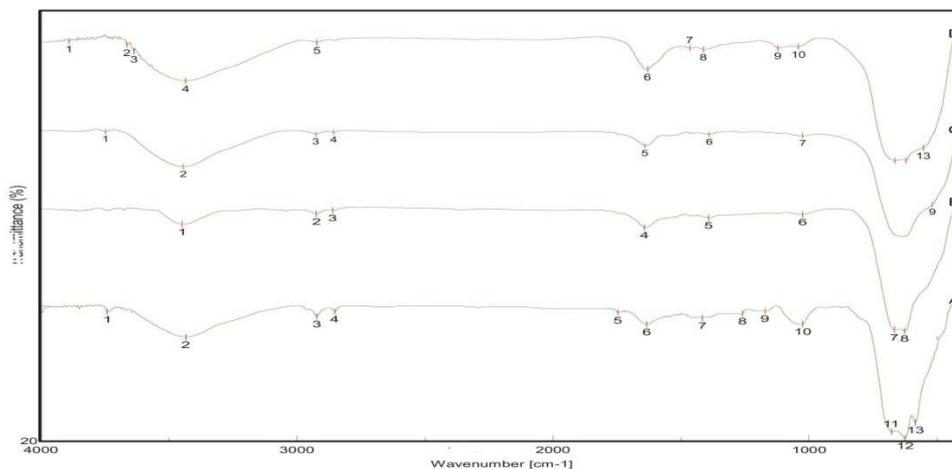
Figure 2. FTIR images of pure (A) and Al doped  $\text{SnO}_2$  (B, C and D)
