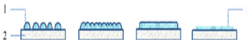
Figure 1. Steps of spray-coating film formation, (1) polymer drops, (2) urea substrate, (3) film layer [1, 18]
