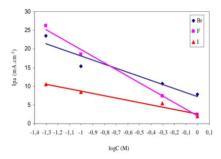
Fig. 4 Evolution of  $I_{pa}$  as function of logarithm of the halogens concentration.
