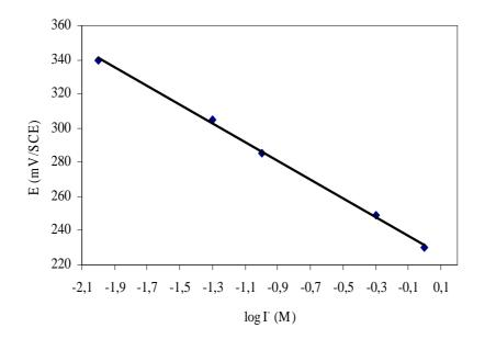
Fig. 5 Variation of  $E_{eq}$  as function of the logarithm of the concentration of the ions I
