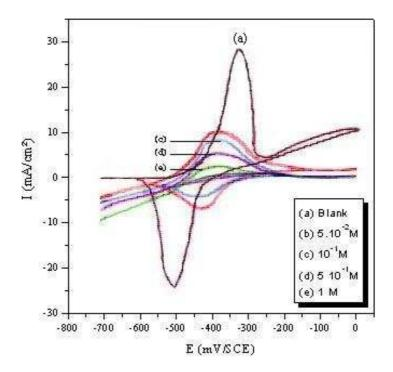
Fig. 3 Cyclic voltammograms for the lead electrode in 0.3M HCl in the presence of I<sup>-</sup> at various concentrations
