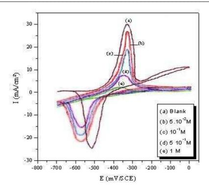
Fig. 2 Cyclic voltammograms for the lead electrode in 0.3M HCl in the presence of F<sup>-</sup> at various concentrations
