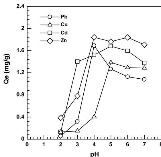
Figure 4: Effect of pH on the uptake capacity of Pb(II), Cu(II), Cd(II) and Zn(II) on non-immobilized. (initial concentration 10 mg/L, particle size is 72  $\mu$ m, bio-sorbent mass is 0.1 g, contact time is 60 min, stirring speed is 150 rpm)
