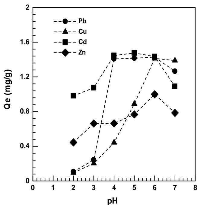
Figure 5: Effect of Ph onthe uptake capacity of Pb(II), Cu(II), Cd(II) and Zn(II) on alginateimmobilization durian seed (gel bead). (Initialconcentration:10mg/L; volume of solution: 20 mL; mass of bio-sorbent: 0.1g; agitation: 120 minutes; stirring speed: 150rpm)
