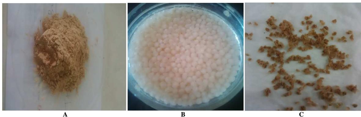
Figure 2: Non immobilized (A), gel(B) and drybead(C) bio-sorbent.
