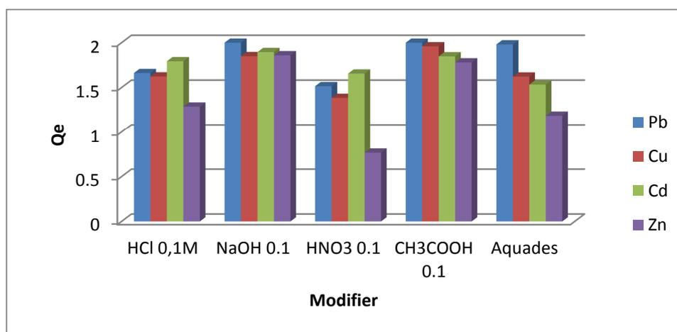
Figure1: Effect of treatment durian seed powder on biosorption of Pb(II), Cu(II), Cd(II) and Zn(II) ions (pH of metals ion was 5, contact time was 60min, agitation speed was 150rpm, mass of bio-sorbent 0.1g and concentration of solution was 10mg/L)
