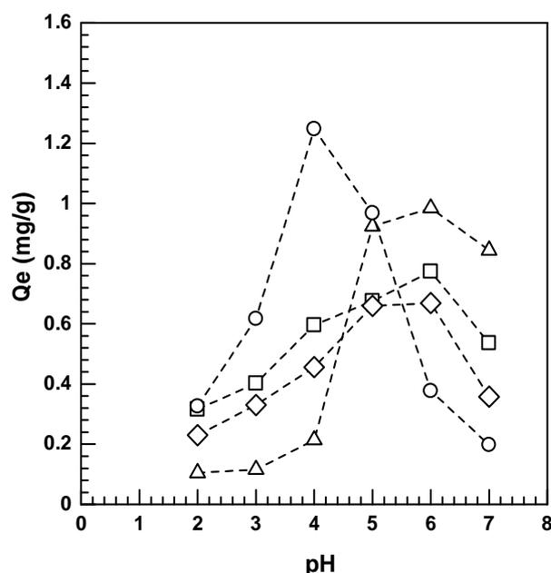
Figure 7: Effect of pH on the uptake capacity of Pb(II), Cu(II), Cd(II) and Zn(II) on Ca-alginate bio-sorbent. (Initial concentration :10mg/L; volume of solution : 20 mL; mass of bio-sorbent : 0.1g; agitation: 120 minutes; stirring speed: 150rpm)
