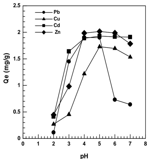
Figure 6: Effect of pH on the uptake capacity of Pb(II), Cu(II), Cd(II) and Zn(II) on alginateimmobilization durian seed (dry bead). (Initial concentration:10mg/L; volume of solution: 20 mL; mass of bio sorbent: 0.1g; agitation:120 minutes; stirring speed: 150rpm)
