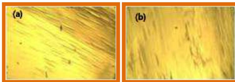
Figure 7. (a) Etch pattern of pure LAM crystal 10 seconds (b) KI doped LAM crystal 10 seconds
