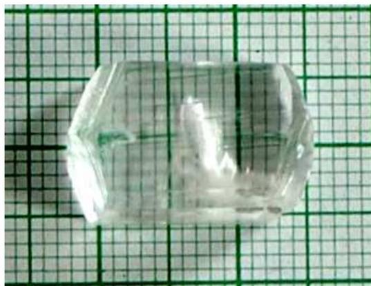
Figure 2. KI - doped LAM crystals
