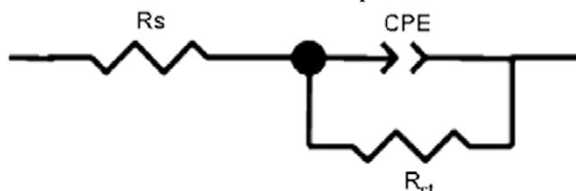
Figure 7: Electrical equivalent circuit used to fit the EIS data of the interface mild steel/1.0 M HCl solution without and with CNEO inhibitor
