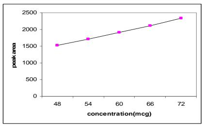
Fig 5: Linearity curve of Nanoxel
