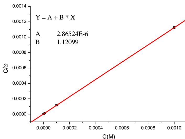
Figure 1. Langmuir adsorption isotherm for P2 on the mild steel surface
