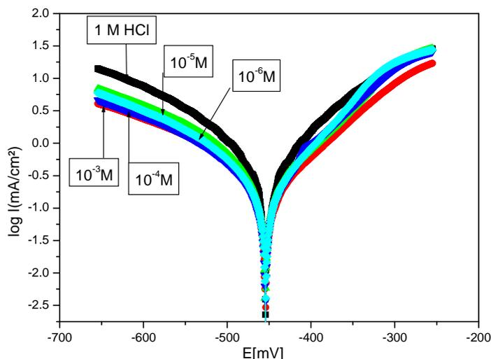
Figure 2. Polarisation curves of mild steel in 1M HCl at different concentrations of P2
