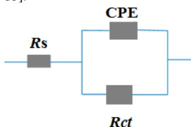
Figure 4. Equivalent circuit model used to fit the impedance spectra
