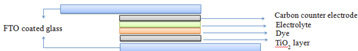
Figure 5: Sandwich type assembly of DSSC
