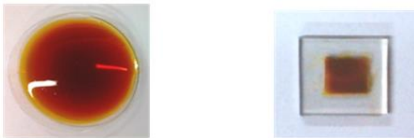
Figure 1: Aqueous solution of Alizarin dye on watch glass and dye absorption on TiO 2 layer coated substrate
