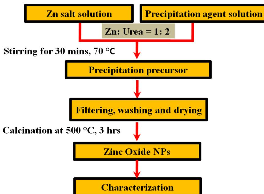
Scheme 1: Chemical reactions to synthesize zinc oxide nanostructure
