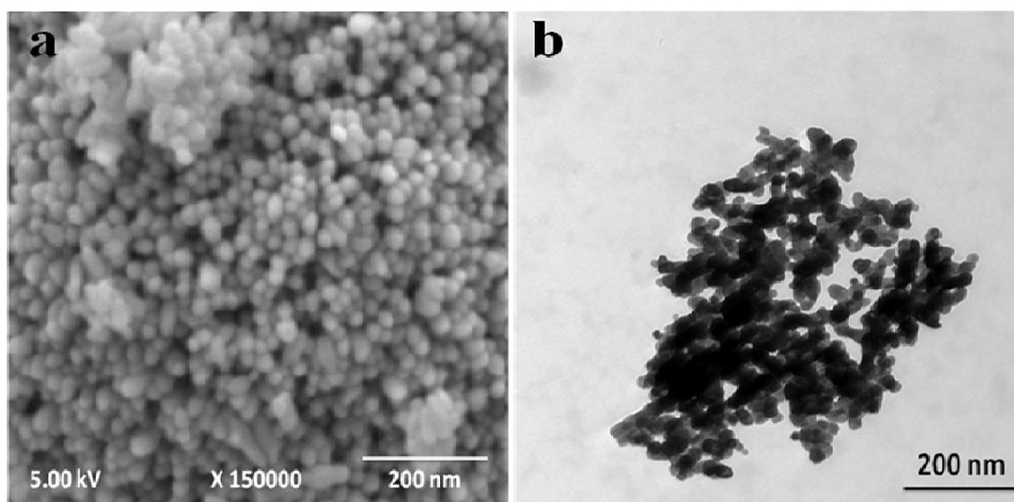
Fig 3. Electron photomicrographs of ZnO nanoparticles (a) SEM image and (b) TEM image
