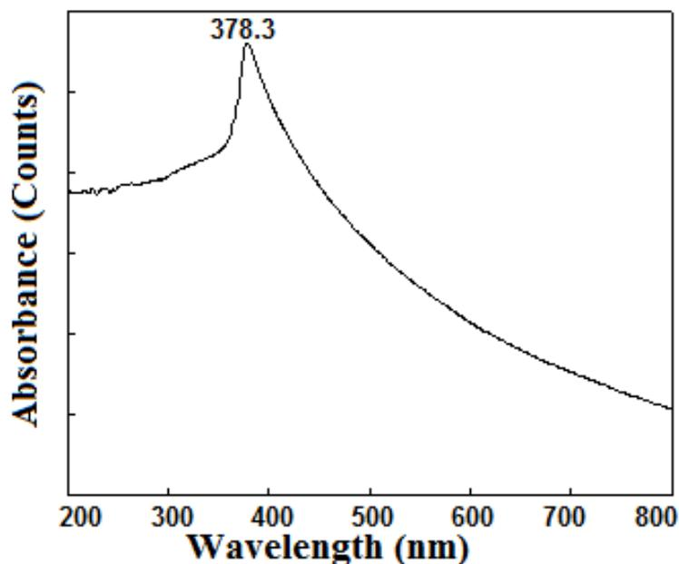
Fig 5. UV-Vis spectra of ZnO obtained from  $0.5\text{ M Zn(NO}_3)_2 \cdot 6\text{H}_2\text{O}$  and  $1\text{ M CO(NH}_2)_2$  calcined at  $500\text{ }^\circ\text{C}$  for 3 hr
