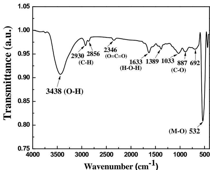
Fig 4. FT-IR spectra of ZnO obtained from  $0.5\text{ M Zn(NO}_3)_2 \cdot 6\text{H}_2\text{O}$  and  $1\text{ M CO(NH}_2)_2$  calcined at  $500\text{ }^\circ\text{C}$  for 3 hr
