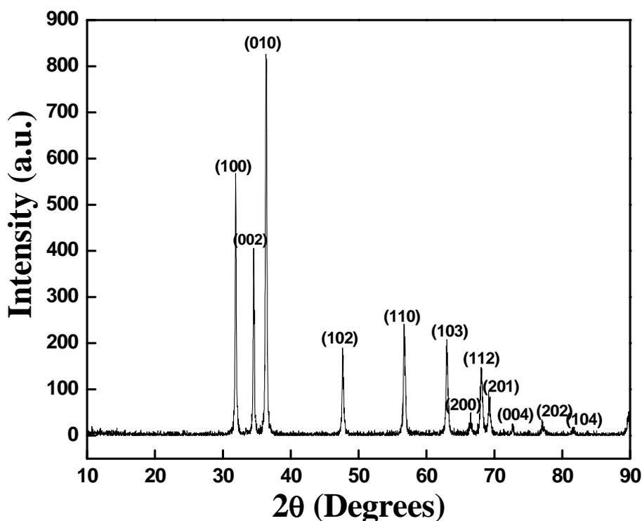
Fig 1. X-ray diffraction patterns of zinc oxide nanoparticles
