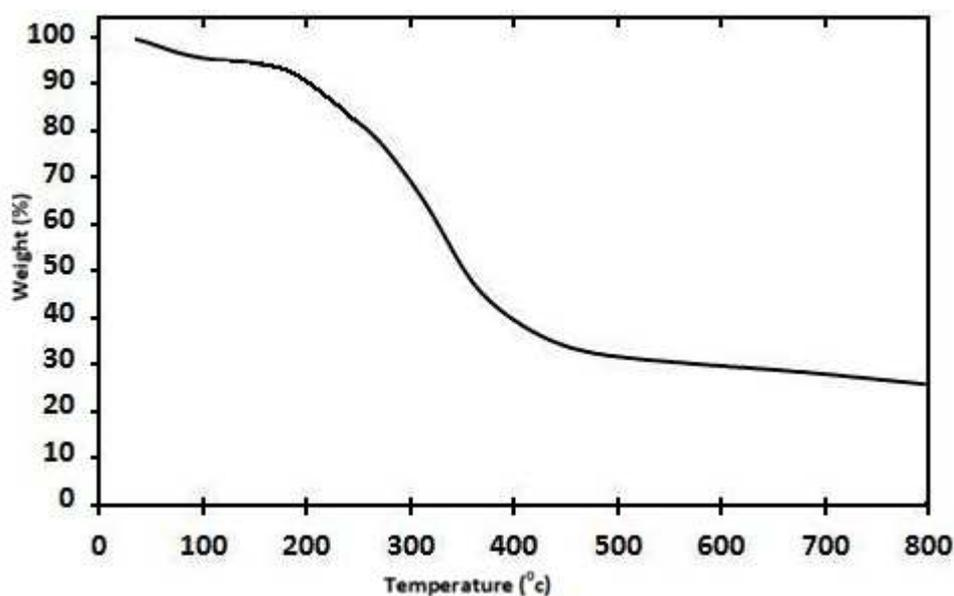
Fig 2. TGA curve of precipitation precursor
