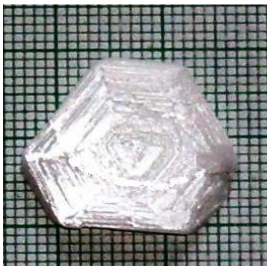
Fig. 1. As grown crystal of Urea Lead Nitrate.
