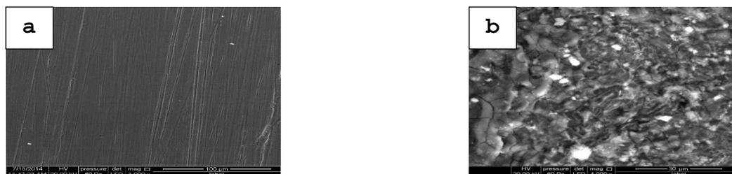
Figure 10: SEM image of mild steel surface (a) before immersion in 1M HCl, (b) after 6 hours of immersion in 1M HCl solution in the absence of inhibitors
