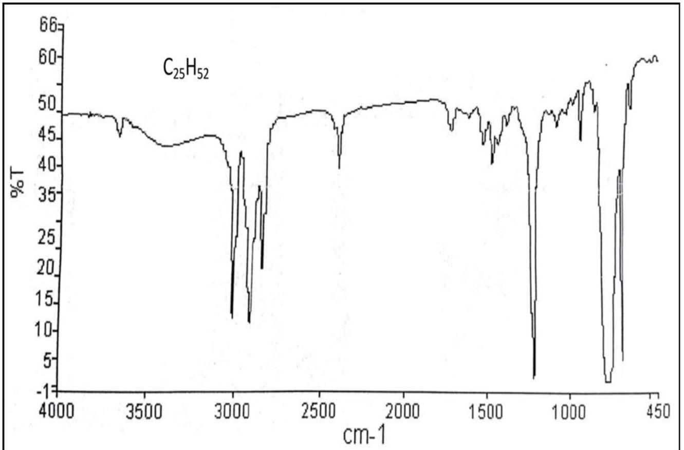
Figure S5: IR spectrum of *n*-Pentacosane (MC-2)
