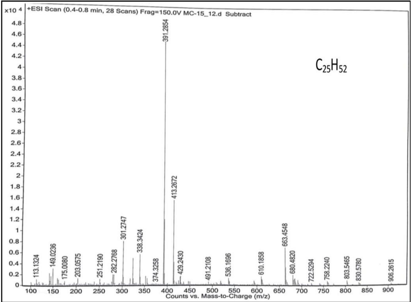
Figure S8: Mass spectrum of *n*-Pentacosane (MC-2)
