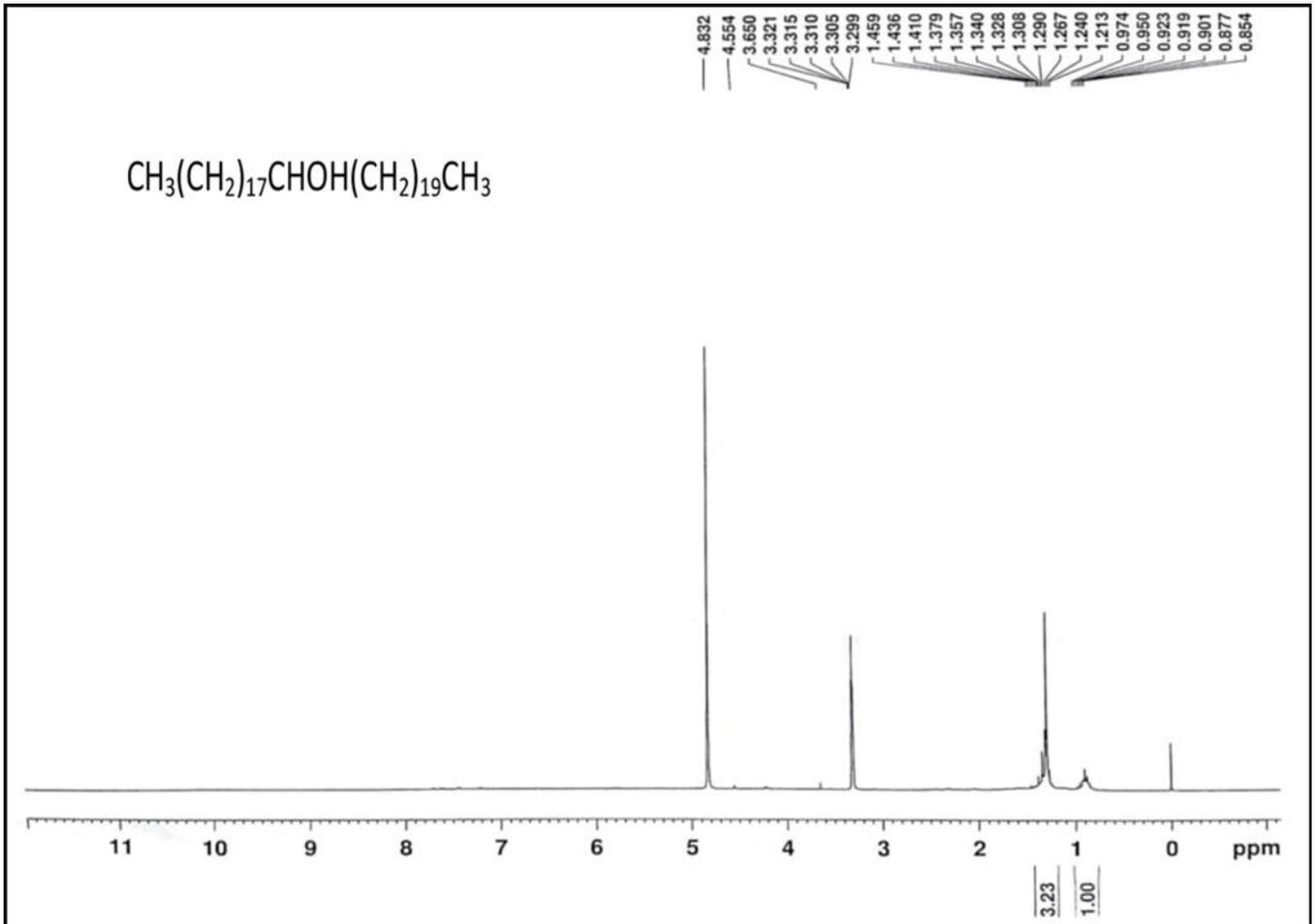
Figure S14:  $^1\text{H-NMR}$  spectrum of *n*-Nonatriacontan-19 $\alpha$ -ol (MC-4)
