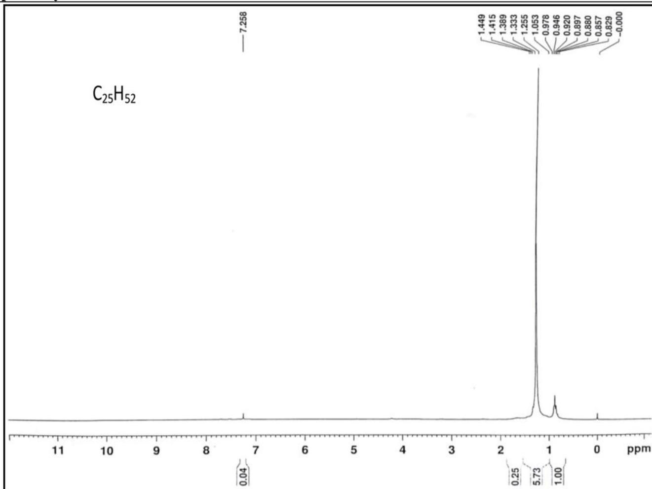
Figure S6:  $^1H$ -NMR spectrum of *n*-Pentacosane (MC-2)
