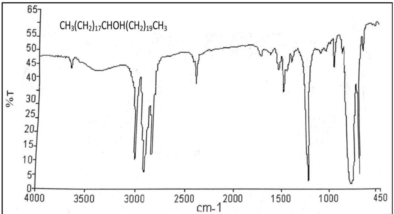
Figure S13: IR spectrum of *n*-Nonatriacontan-19 $\alpha$ -ol (MC-4)
