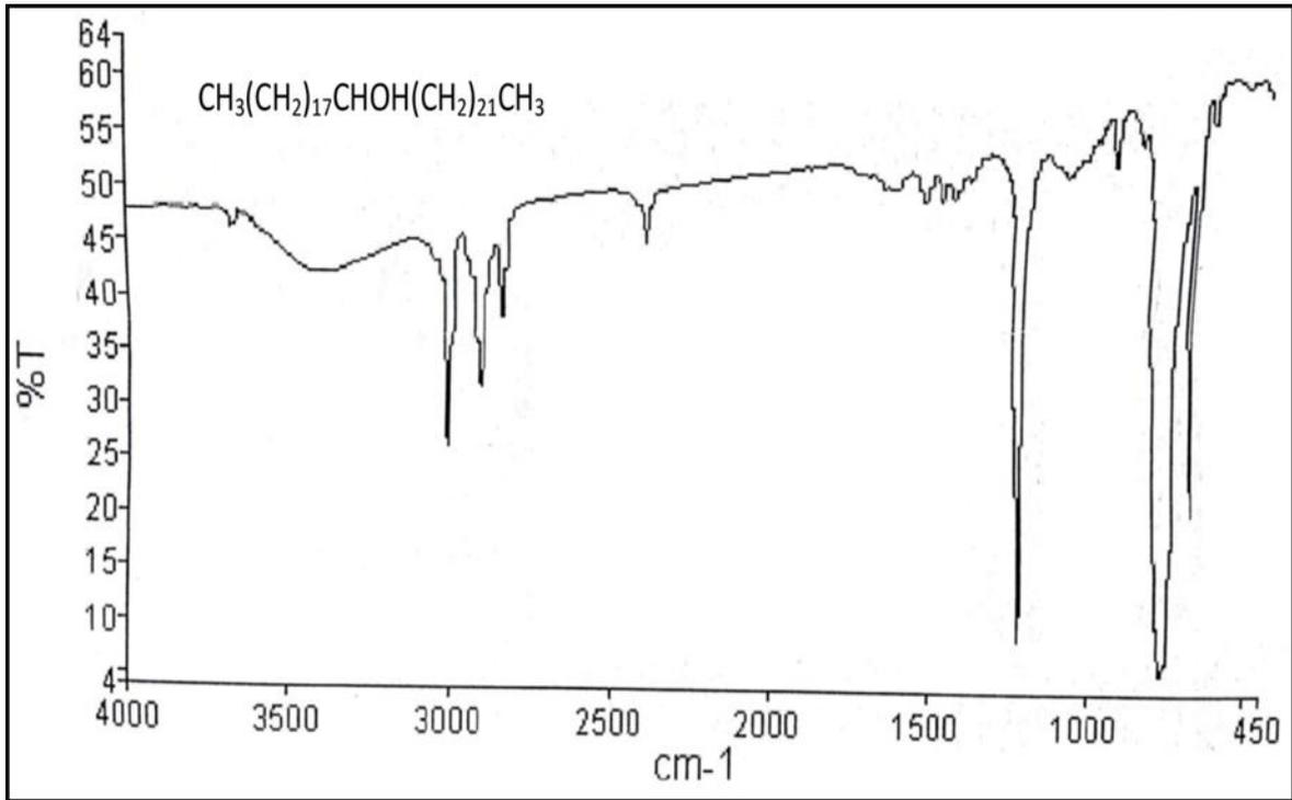
Figure S16: IR spectrum of *n*-Henetracontan-19 $\alpha$ -ol (MC-5)
