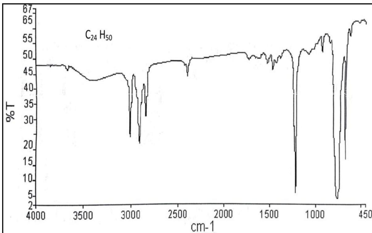
Figure S1: IR spectrum of *n*-Tetracosane (MC-1)
