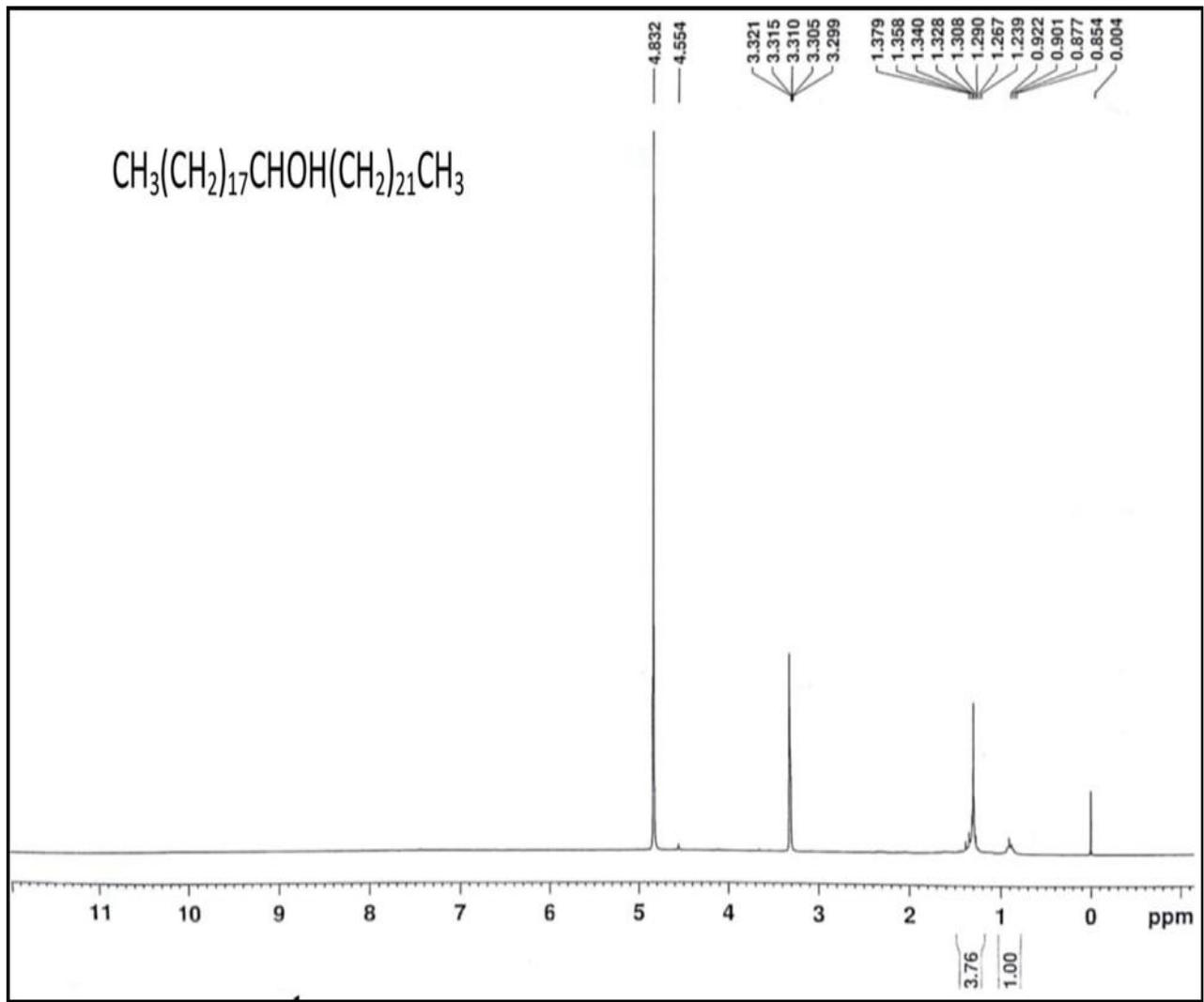
Figure S17: <sup>1</sup>H-NMR spectrum of *n*-Henetracontan-19 $\alpha$ -ol (MC-5)
