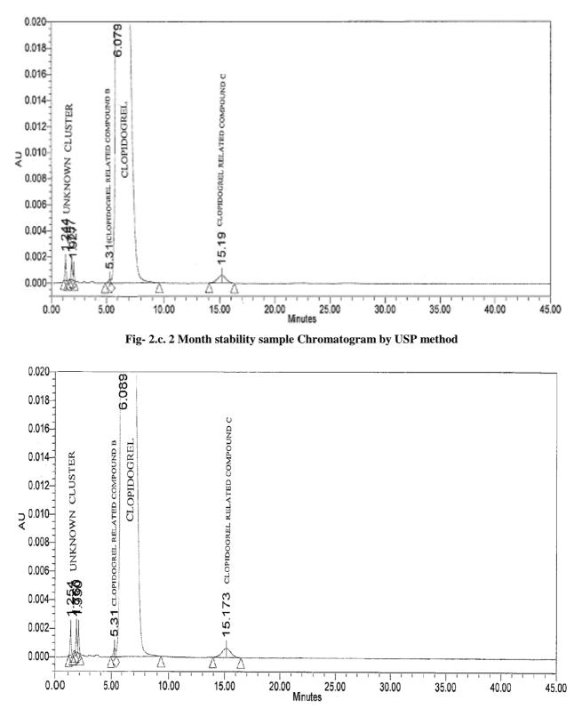
Fig- 2.d. 3 Month stability sample Chromatogram by USP method
