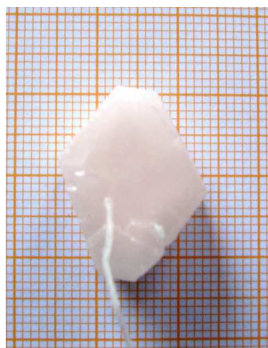
Fig.2 As grown crystal of PTC
