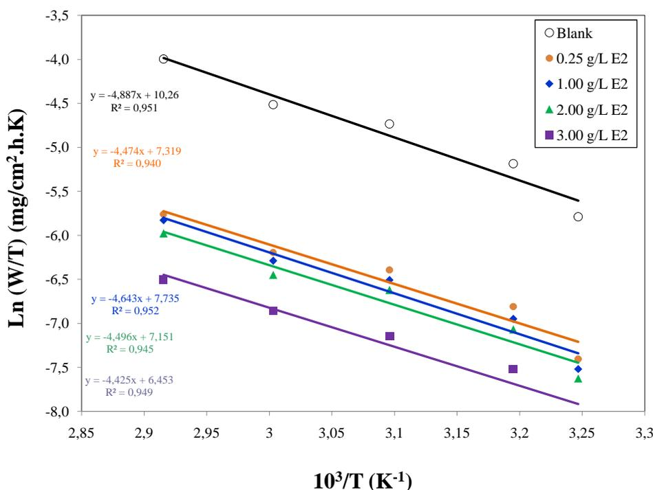
Fig. 9. Transition-state plot for C38 steel corrosion rates (W) in 1 M HCl without and with different concentrations of E2
