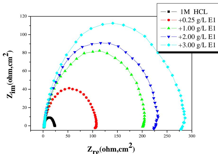
Fig. 3. Nyquist plots for C38 steel in 1 M HCl with various concentrations of E1
