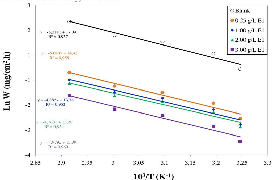
Fig. 6. Arrhenius plots for C38 steel corrosion rates (W) in 1 M HCl without and with different concentrations of E1
