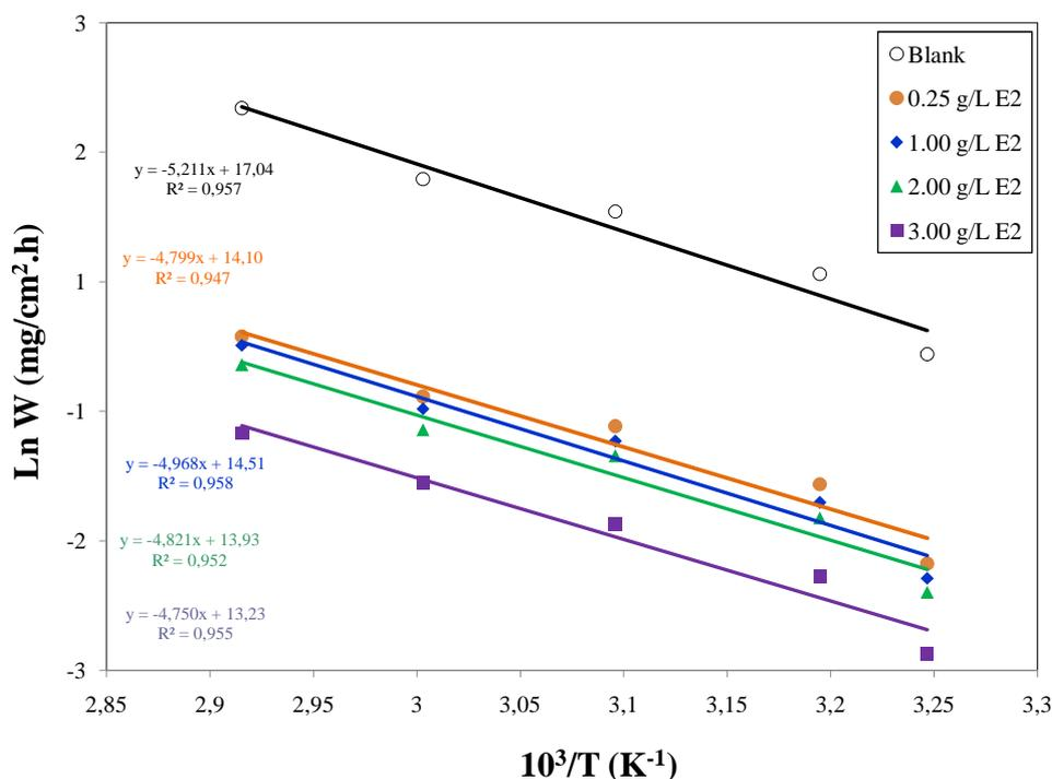
Fig. 7. Arrhenius plots for C38 steel corrosion rates (W) in 1 M HCl without and with different concentrations of E2
