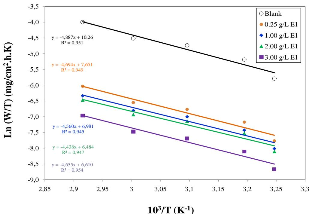
Fig. 8. Transition-state plot for C38 steel corrosion rates (W) in 1 M HCl without and with different concentrations of E1
