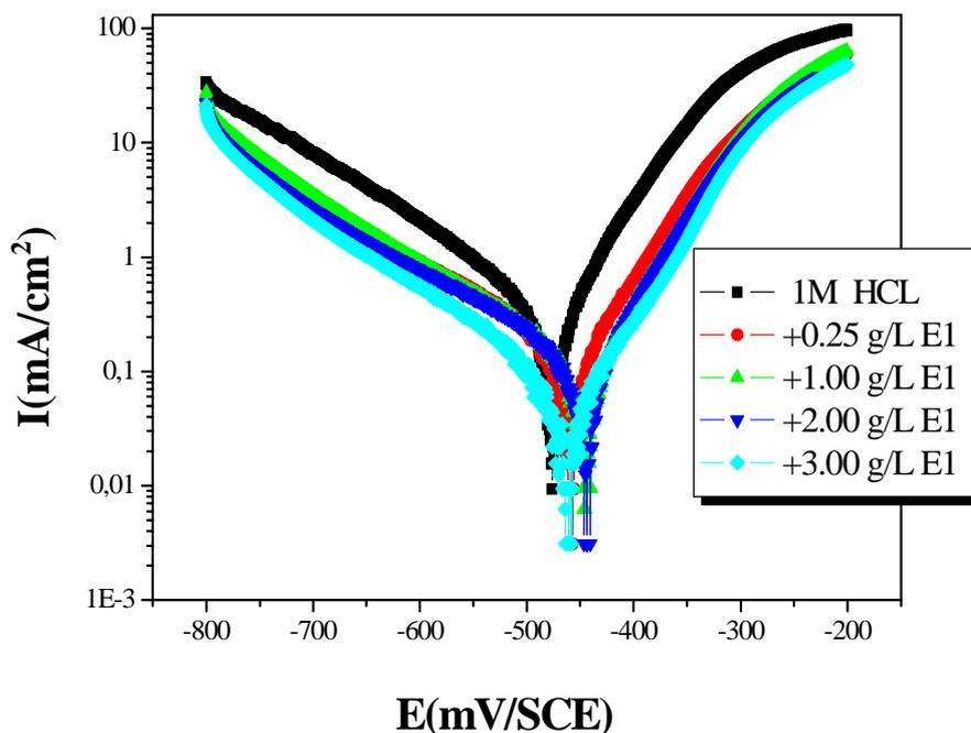
Fig. 1. Anodic and cathodic polarization curves of C38 steel in 1 M HCl with various concentrations of E1
