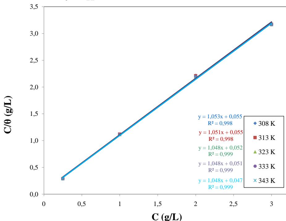
Fig. 10. Langmuir adsorption isotherm of E1 on the C38 steel surface in 1 M HCl
