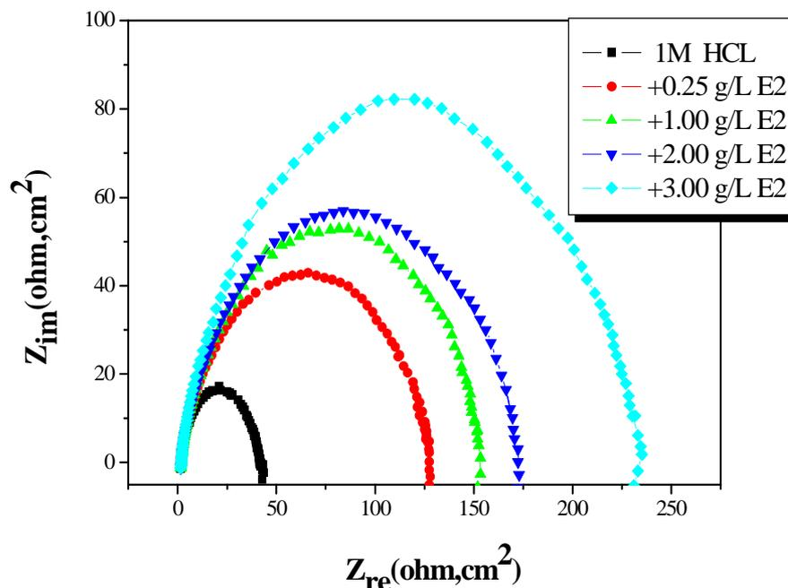
Fig. 4. Nyquist plots for C38 steel in 1 M HCl with various concentrations of E2
