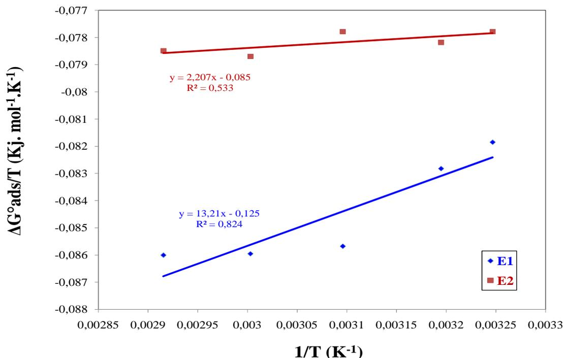
Fig. 13. The relationship between ( $\Delta G^{\circ}_{ads}/T$ ) and  $1/T$  of E1 and E2
