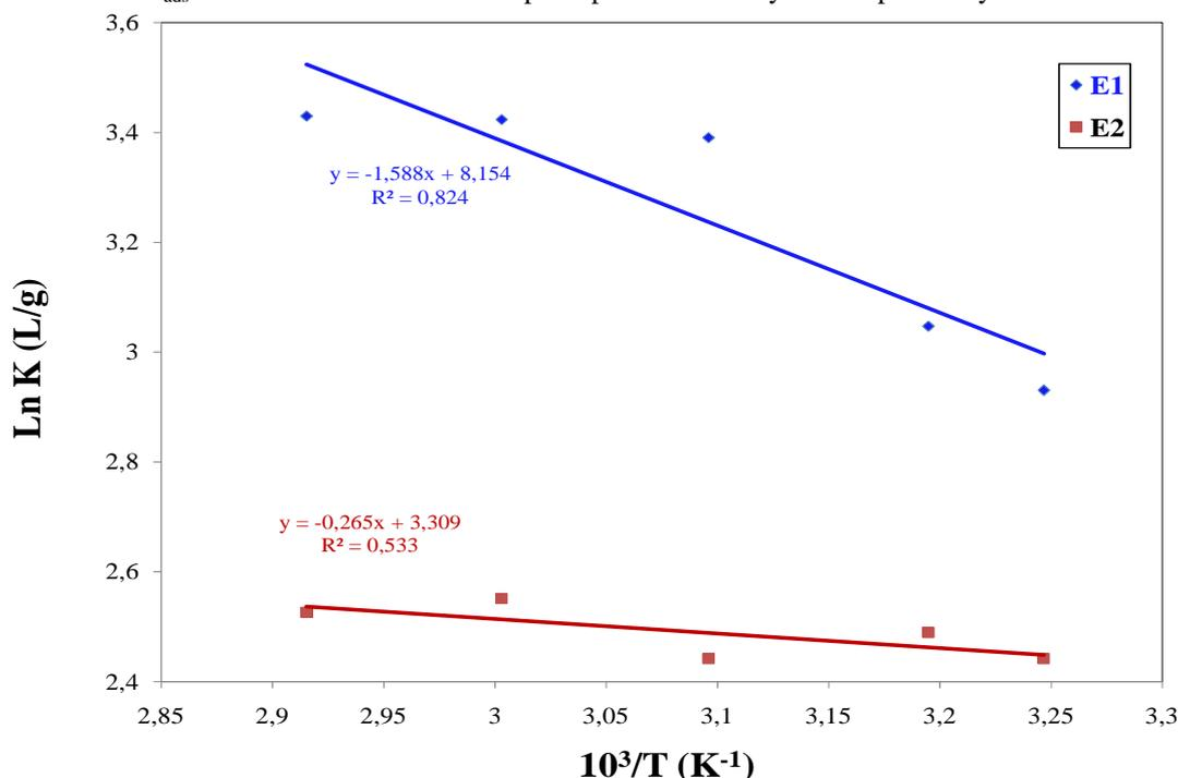
**Fig. 12.** Van't Hoff's plot of Ln K against  $1/T$  for the adsorption of E1 and E2 onto C38 steel
