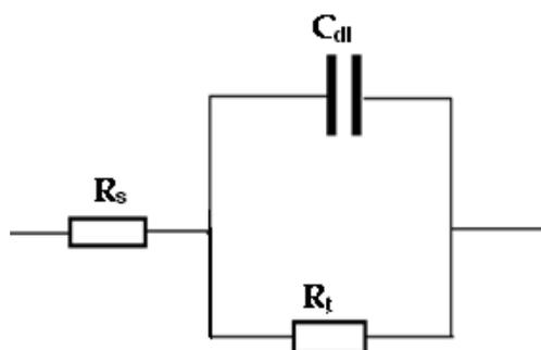
Fig. 5. Equivalent circuit used to fit the EIS data of C38 steel in 1 M HCl without and with different concentrations of aqueous extract from *A. leucotrichus* fruits (E1 and E2)
