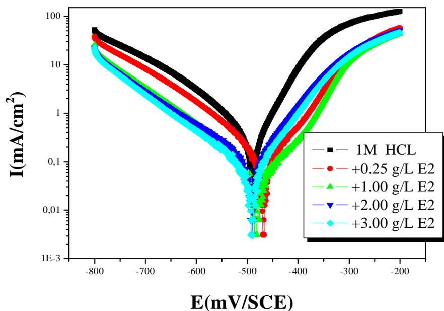
Fig. 2. Anodic and cathodic polarization curves of C38 steel in 1 M HCl with various concentrations of E2
