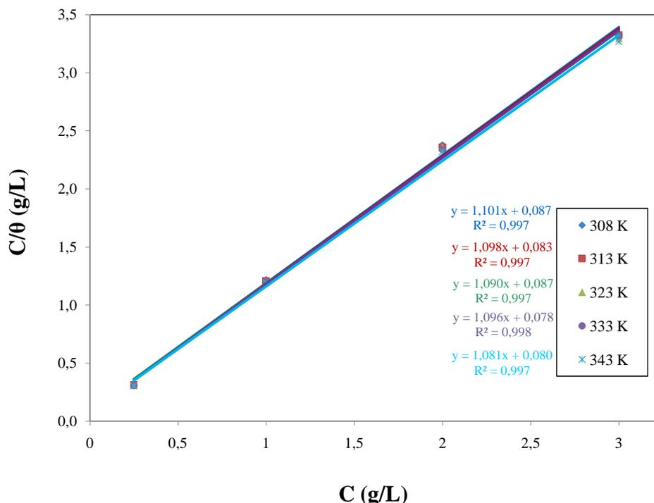
Fig. 11. Langmuir adsorption isotherm of E2 on the C38 steel surface in 1 M HCl
