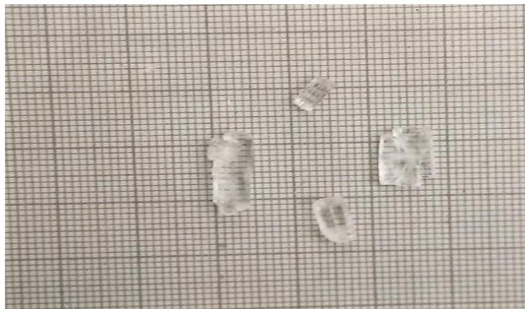
**Fig 2. Diagram of as grown ZBdM crystal**
