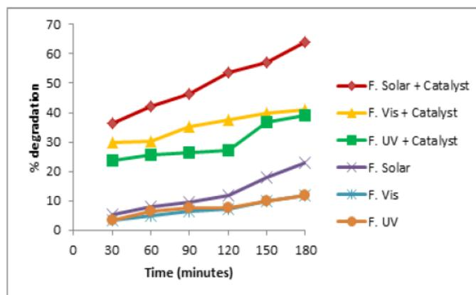
Figure 6: Effect of light sources in photolysis and photocatalytic processes of orange F3R
