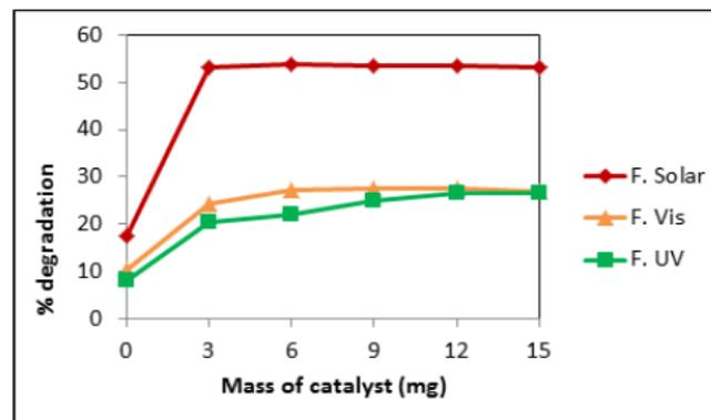
Figure 4: Effect of catalyst loading under different light sources
