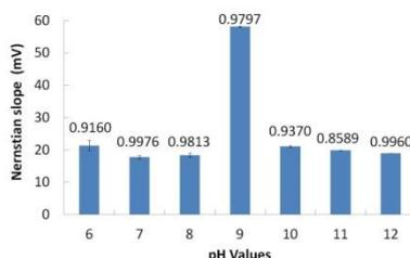
Figure 4: Nernstian response for ionophore (1) over a range of pH values with their associated correlation coefficients (n=3 and error bars (where visible) indicate the standard deviation)
