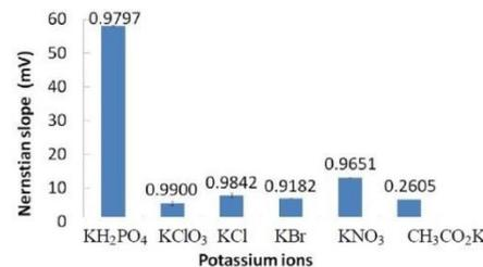
**Figure 5: Nernstian response for ionophore (1) against a range of potassium ions with their associated correlation coefficients ( $n=3$  and error bars (where visible) indicate the standard deviation)**
