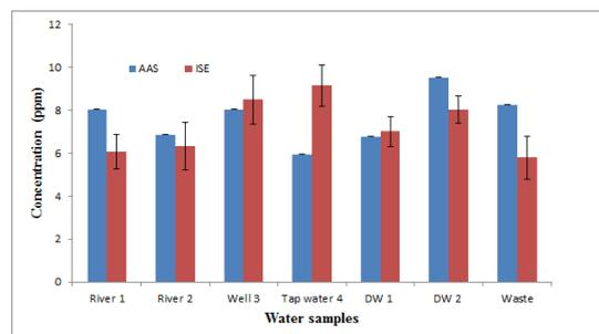
**Figure 6: Water samples measurements for ionophore (1) in ISE method with comparison with AAS method ( $n=3$  and error bars (where visible) indicate the standard deviation)**
