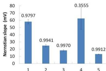
Figure 3: Nernstian response for a range of ionophores with their associated correlation coefficients (n=3 and error bars indicate the standard deviation)
