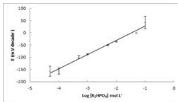
**Figure 2: Potential response of the potassium ISE containing ionophore (1) vs. Ag/AgCl reference electrode for increasing concentrations of potassium phosphate ion at pH 9 (n=3 and error bars (where visible) indicate the standard deviation)**
