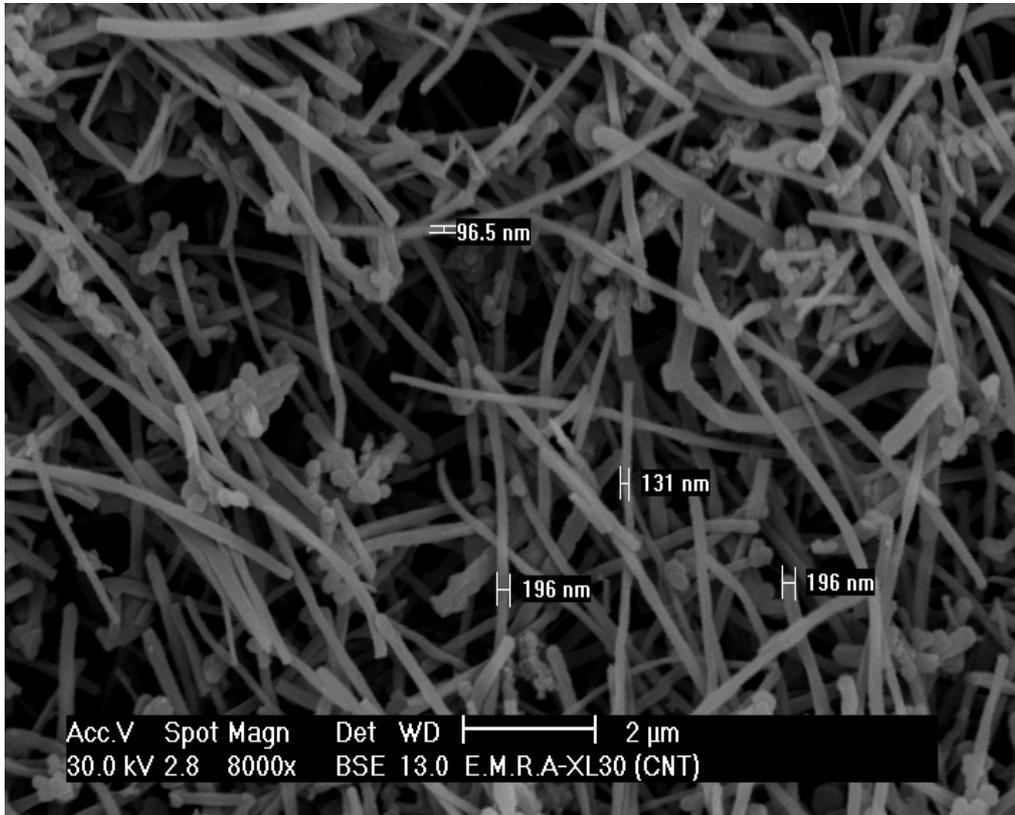
**Fig( 1 ):** SEM image of multi-walled carbon nanotube MWCNT.
