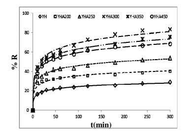
Fig 2. adsorption kinetics of MB molecule by YHAx (x : activation temperature)
