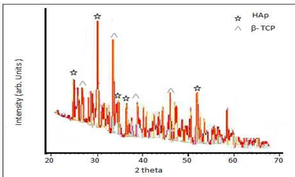
Figure 5. X-ray diffraction of the cured cement after hydrolysis and calcination at 900 ° C
