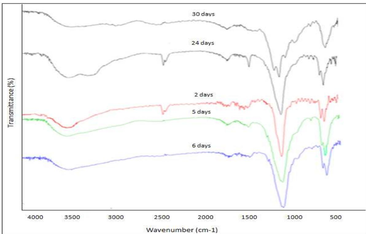
Figure 2. IR spectra of the cured cement evolution, in a solution of  $H_2O_2$  at pH =10
