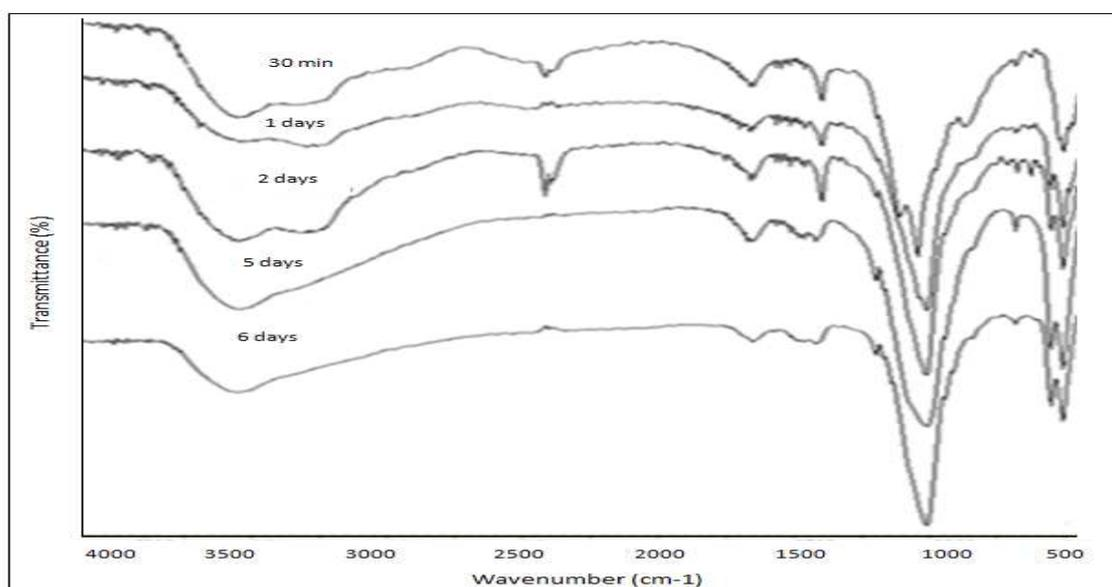
Figure 3. Infrared spectra of the evolution of the cement hardened in a solution of  $H_2O_2$  at pH = 11
