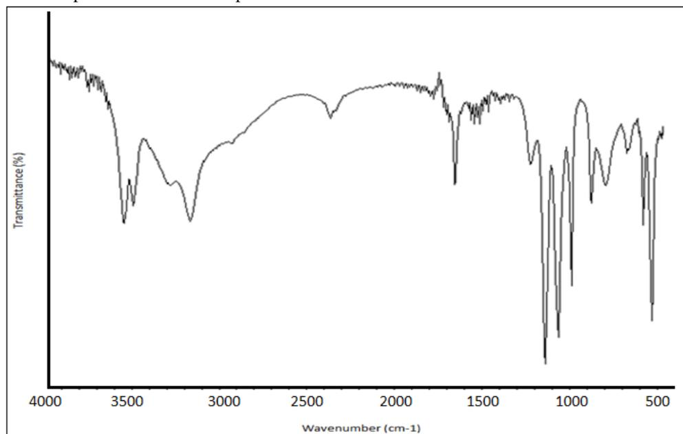
Figure 1. Infrared spectrum of the cured cement
