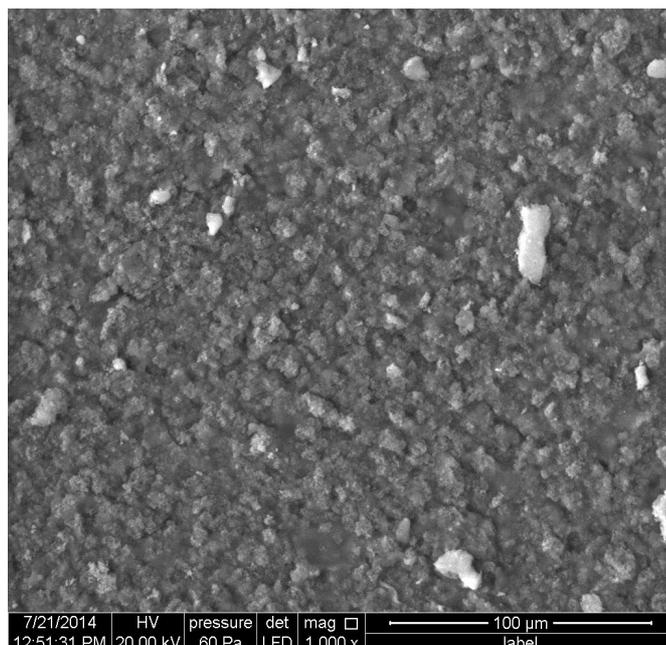
Figure 6. Transmission microscopy of the cured cement after hydrolysis at pH = 10
