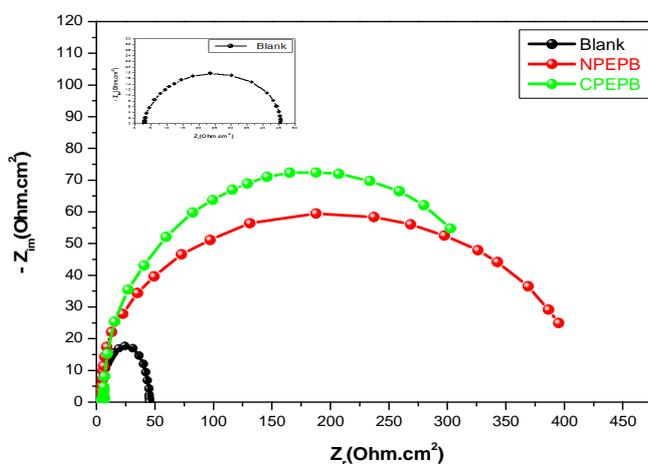
Fig 2: Nyquist diagrams for copper electrode in (2M H<sub>3</sub>PO<sub>4</sub>+ 0.3M NaCl) in absence and presence of optimum concentration 10<sup>-3</sup>M of inhibitors (NPEPB and CPEPB)
