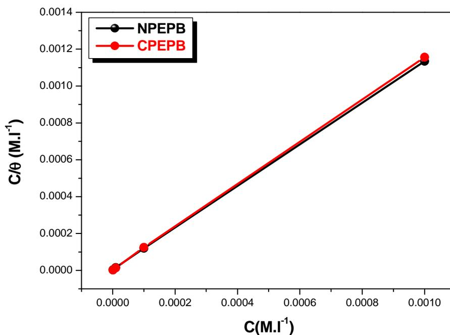
Fig.5: Plots of Langmuir adsorption isotherm in the presence of NPEPB and CPEPB on the Copper surface at 298K
