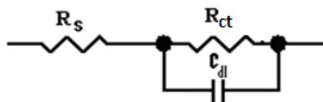
Fig. 3 The electrochemical equivalent circuit used to fit the impedance spectra
