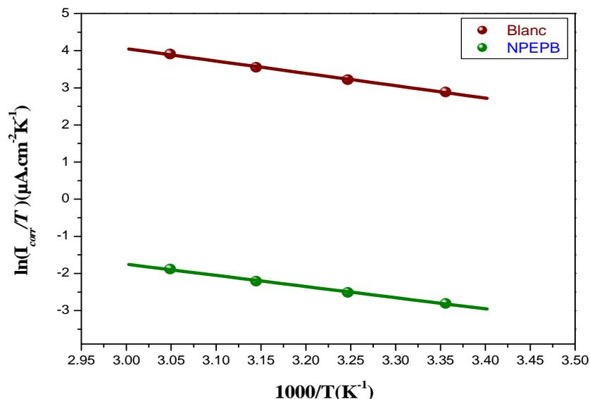
Fig 11. Relation between  $\ln(I_{corr}/T)$  and  $1000/T$  at different temperatures
