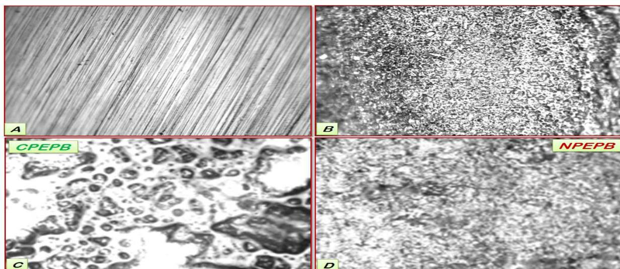
Fig. 11. OM (x200) of tinplate (A) before immersion (B) after 6h of immersion of copper in phosphoric acid (C and D) after 6h of immersion in 2M H<sub>3</sub>PO<sub>4</sub>+0.3M NaCl +10<sup>-3</sup>M of CPEPB and NPEPB at 298K
