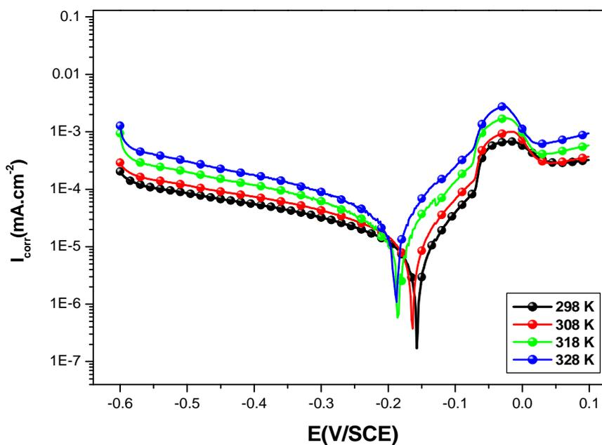
Fig 9 : Potentiodynamic polarization curves of Copper in 2M H<sub>3</sub>PO<sub>4</sub> + 0.3M NaCl in the presence of 10<sup>-3</sup> M of NPEPB at different temperatures
