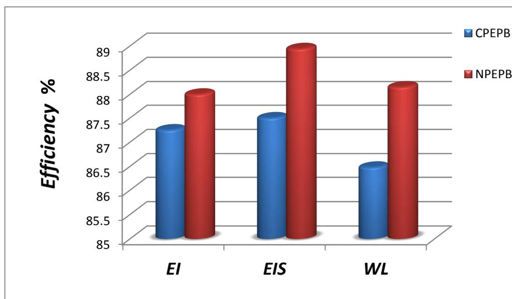
**Fig.6: Comparison of inhibition efficiency (E %) values obtained by weight loss, polarization and EIS methods at optimum concentration 10<sup>-3</sup>M of inhibitors (NPEPB and CPEPB)**
