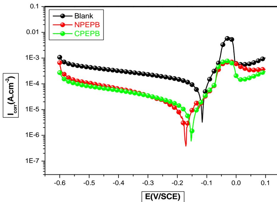
Fig 1. Potentiodynamic polarization curves of Copper in (2M H<sub>3</sub>PO<sub>4</sub> + 0.3M NaCl) in absence and presence of optimum concentration of NPEPB and CPEPB at 298 K
