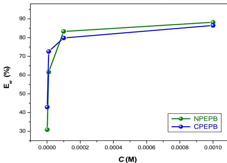
Fig.4. Variation of the inhibition efficiency ( $E_w$  %) of Copper corrosion with the concentration of NPEPB and CPEPB in 2M  $H_3PO_4$  + 0.3M NaCl at 298 K
