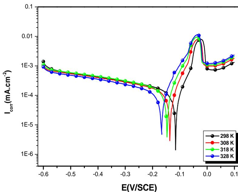
Fig 8 : Potentiodynamic polarization curves of copper in (2M H<sub>3</sub>PO<sub>4</sub> + 0.3M NaCl) at different temperatures
