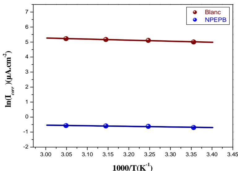
**Fig 10: Arrhenius plots of Copper in 2M H<sub>3</sub>PO<sub>4</sub> + 0.3M NaCl with and without  $10^{-3}$  M of NPEPB**
