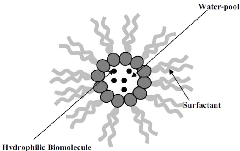
Figure 2: Structure of a reverse micelle [Adapted From: 12]
