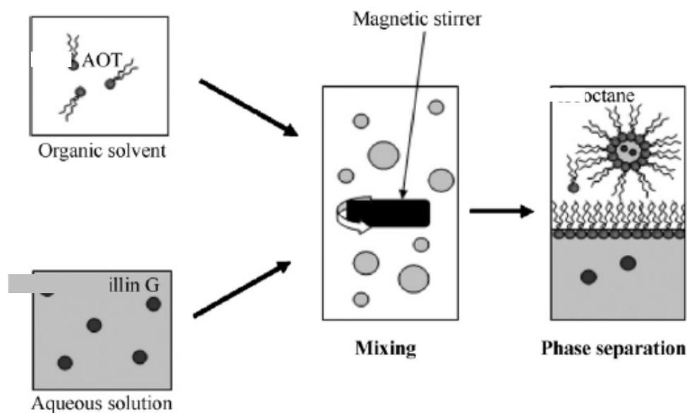
Figure 3: Forward extraction procedure [Adapted From: 27]
