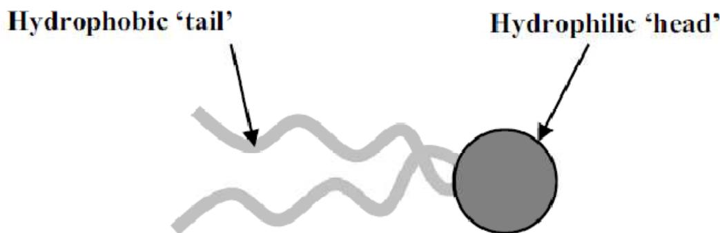
Figure 1: Schematic of a surfactant molecule [Adapted From: 12]
