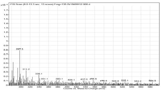
Fig 5 (b): LC-MS spectrum of Complex 3 (280-600 m/z)
