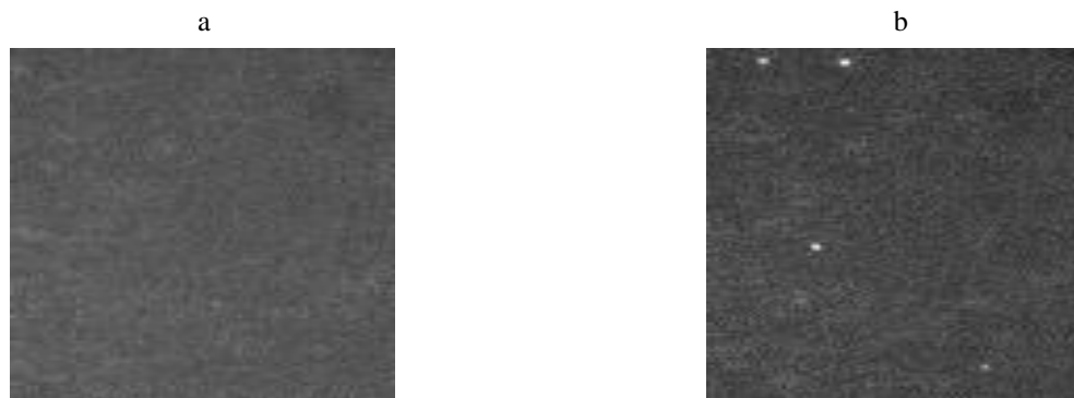
Figure 3 Glass slides test with only mounting solution a) non-autofluorescent glass slide. b) It is clear the bright spots resulting from the autofluorescent of the rare earth particles in the glass slide.
