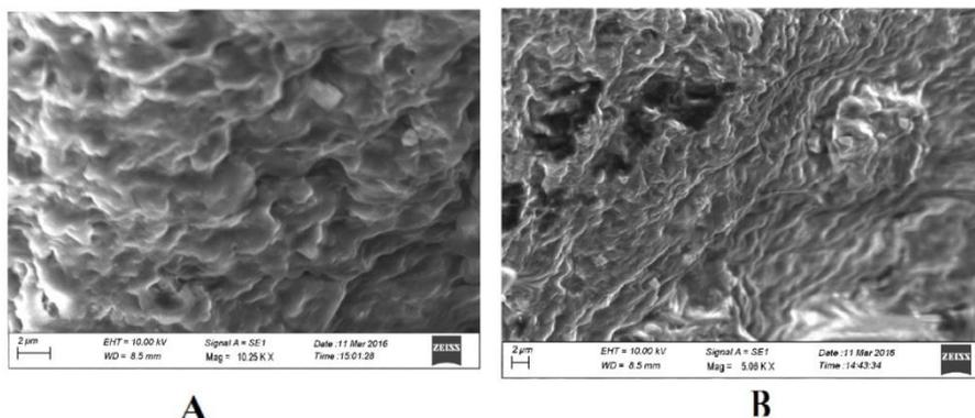
**Figure 2: (A) PFB SEM image, (B) PFB loaded with simvastatin SEM image**
