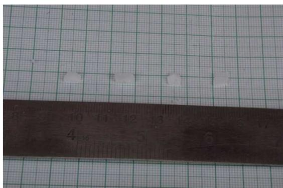
Fig. 1.2 Photographs of as grown  $\text{Cd}^{2+}$  doped BTMC single crystals
