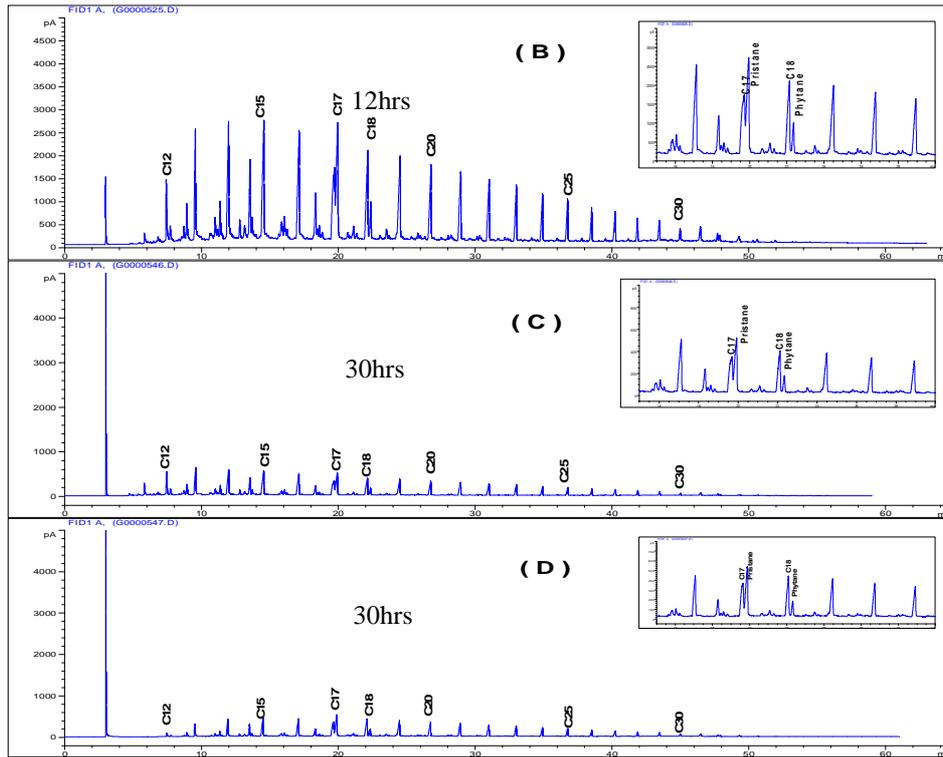
Fig. (2): Gas chromatograms of the Control (undegraded) and degraded samples using *S.rosinii* before irradiation (A and C) and after irradiation (B and D) at two incubation times.
