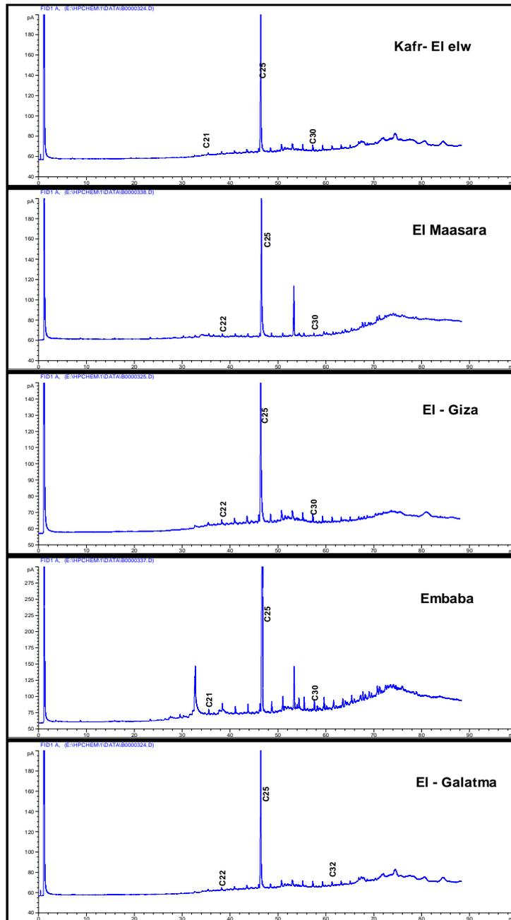
Fig. (1): Gas chromatograms of the extracted hydrocarbons in the collected water samples from the five studied sites along the River Nile.
