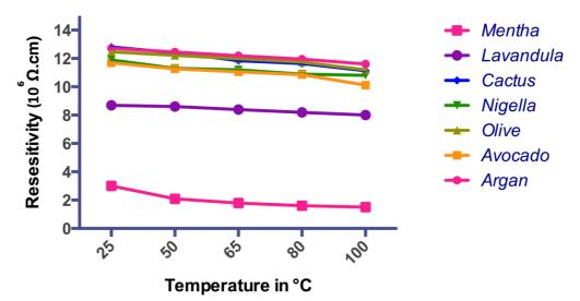
Figure 1: Electrical resistivity of vegetable and essential oils
