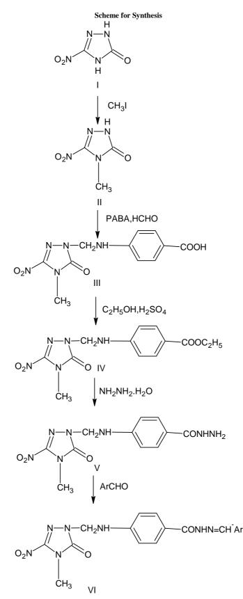
Synthesis of 5-nitro-2,4-dihydro-3H-1,2,4-triazol-3-one (nitration): Nitric acid (90ml) was added to the (10g) of triazolone marinating the temperature between 0°C to 5°C. The mixture was heated to 60-70°C with constant stirring .The reaction was exothermic and brown fumes were evolved. After sometime mixture was chilled (0 to 5°C) in an ice-bath, filtered and washed with water to remove excess nitric acid. Pure nitrotriazolone was crystallized by water. Yield 80% [10].
