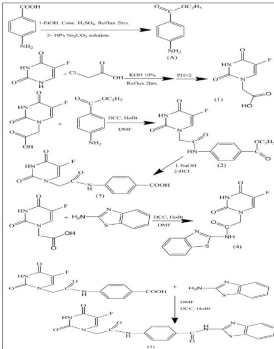
Scheme 1: The synthetic pathway of the intermediate and final target compounds
