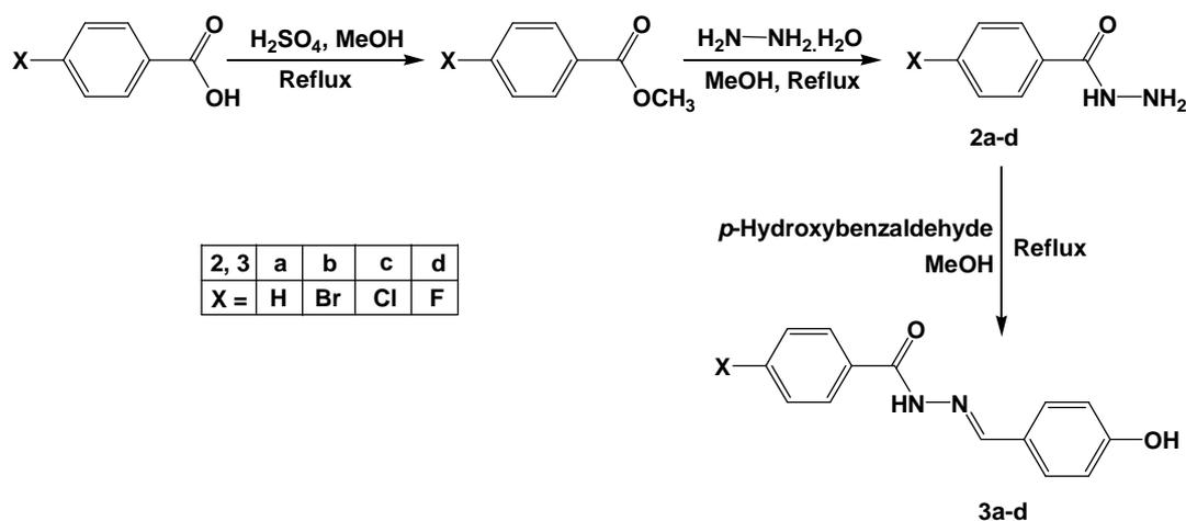
**Scheme 1. Synthesis of 4-substituted *N'*-(4-hydroxy-benzylidene)-hydrazides**
