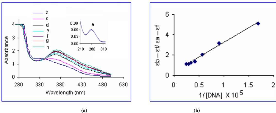
Figure 2. (a). UV-Visible spectra of RuP complex with and without mixing CT-DNA at different concentrations, along with simple CT-DNA and (b). plot of  $\epsilon_b - \epsilon_f / \epsilon_a - \epsilon_f$  against reciprocal of concentration of CT- DNA ( $1/[DNA]$ ).
