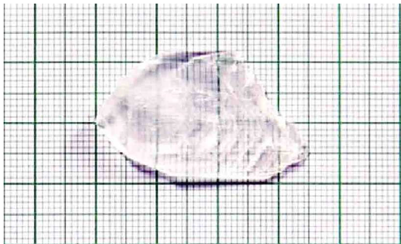
Fig. 2 Photograph of as grown ULMA crystal
