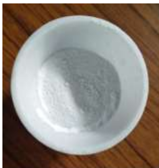
Figure 1: Calcium oxide obtained from calcination of chicken eggshells at 900°C.
