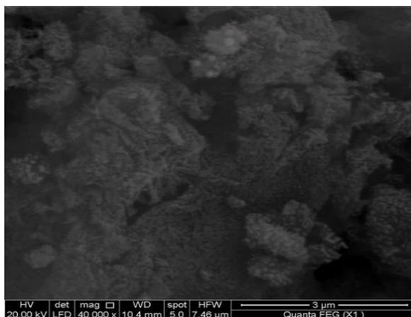
Figure 3d: FESEM image of *Bacillus* -H-Titanate Nanotubes Composite (BT-TNT)
