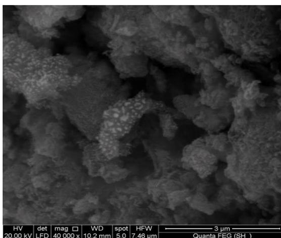
Figure 3c: FESEM image of multilayered H-Titanate Nanosheets (TNS)
