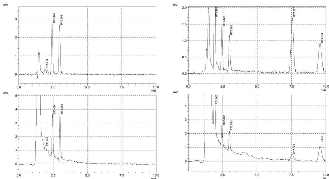
Fig. 1. HPLC-UV response obtained in dual mode; 325 nm (left) and 292 nm (right) after injecting: a standard solution (top chromatograms) and a treated plasma sample (Bottom chromatograms). Identified peaks: BHT ( $t_R = 1.9$  min), Retinol ( $t_R = 2.4$  min), Retinyl acetate ( $t_R = 3.0$  min), tocopherol ( $t_R = 7.5$  min), tocopheryl acetate ( $t_R = 9.5$  min).
