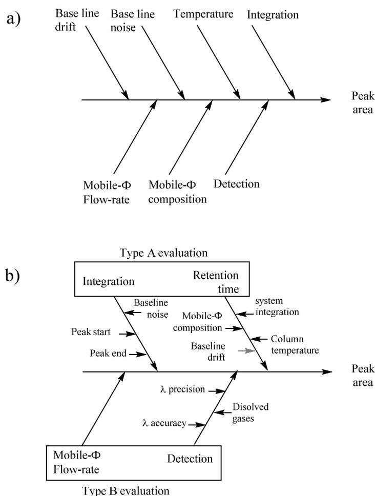
**Fig. 1. Identified sources of uncertainty during the chromatographic assays: a) the main influent factors, b) The same identified effects rearranged according the uncertainty estimation type**
