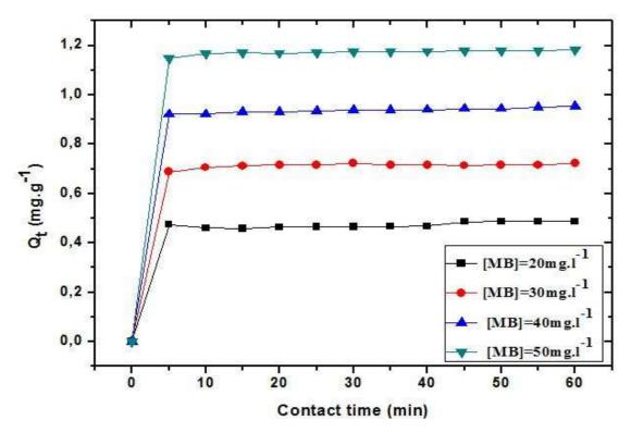
Figure 5: Effect of the contact time on the ER (%) of the MB
