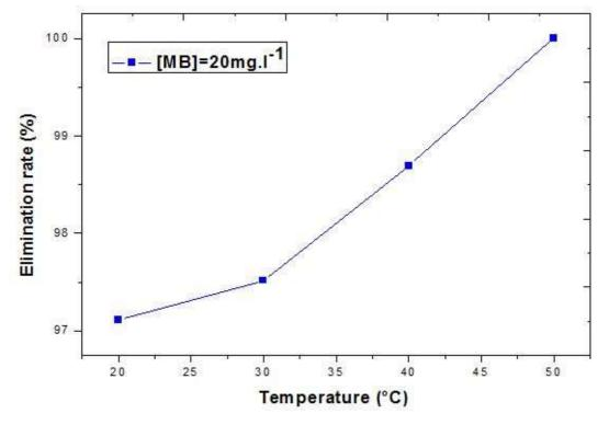
$\label{eq:Figure 10: Effect of temperature on ER (\%)} m=2~g.l^{-1}, MB=20~mg.l^{-1}, T=20-50^{\circ}C, pH=6, V_{steering}=400~tpm ~and ~agitation ~time~60~min$
