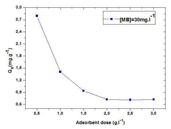
Figure 6: Effect of adsorbent dose (PB) on the  $Q_{ads~(\acute{e}q)}$ . m=0.5-3 g.l<sup>-1</sup>, MB=30 mg.l<sup>-1</sup>, T=20°C, pH=6,  $V_{steering}$ =400 tpm and agitation time 60 min
