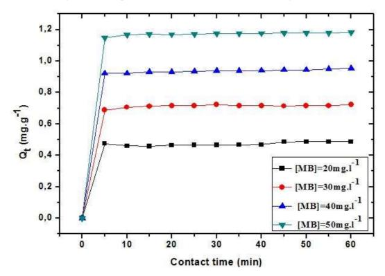
Figure 4: Effect of contact time and MB dye concentration
