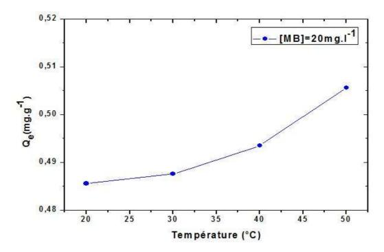
$\label{eq:Figure 9: Effect of temperature on $Q_{ads\ (\acute{e}q)}$} m=2\ g.l^{-1}, MB=20\ mg.l^{-1}, T=20-50^{\circ}C,\ pH=6,\ V_{steering}=400\ tpm\ and\ agitation\ time\ 60\ min$
