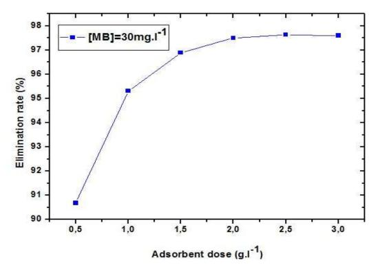
Figure 7: Effect of adsorbent dose (PB) on the ER (%) m=0.5-3 g.l $^{-1}$ , MB=30 mg.l $^{-1}$ , T=20 $^{\circ}$ C, pH=6, V<sub>steering</sub>=400 tpm and agitation time 60 min
