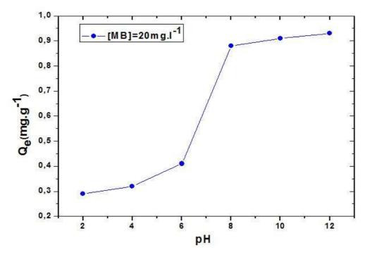
Figure 8: Effect of pH on adsorbed quantity of MB onto PB
