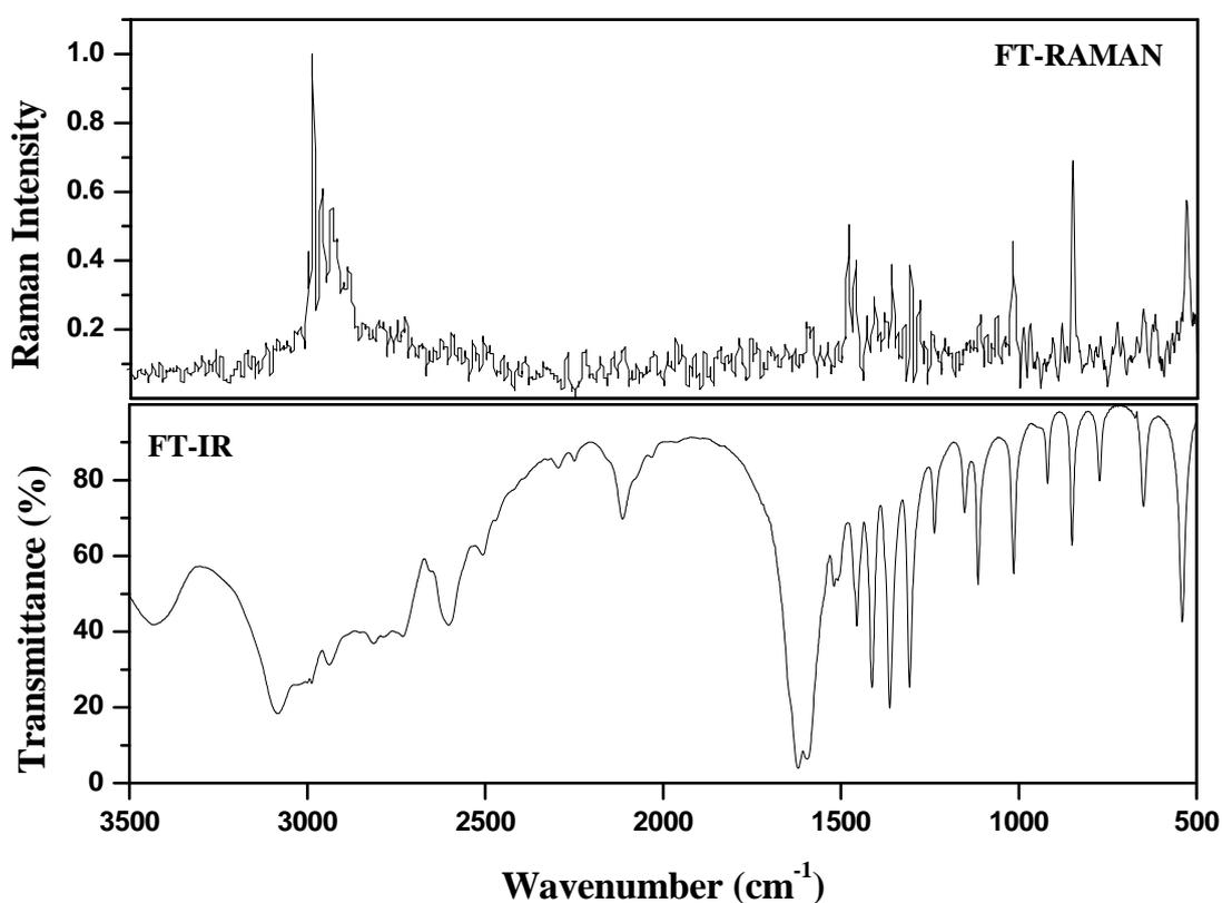
**Fig.2. FT- Raman and FT-IR spectra of LAIA single crystal**
