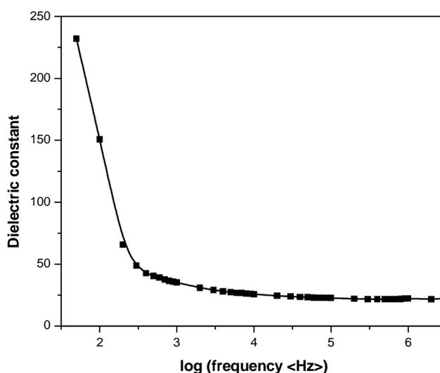
Fig 6 Plot of dielectric constant versus log frequency
