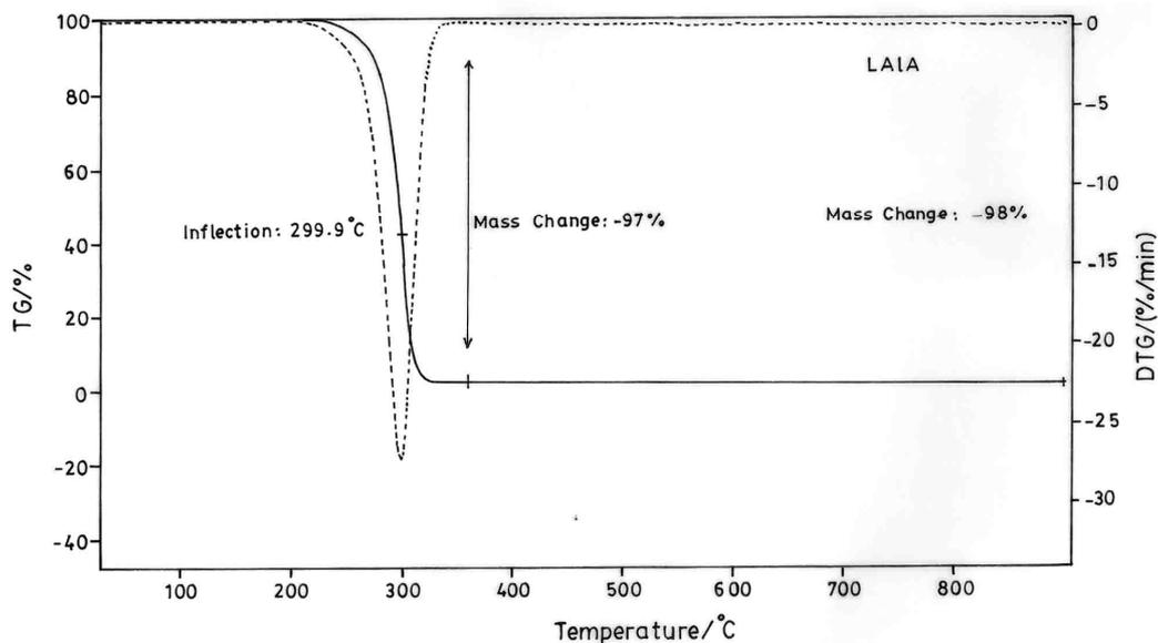
Fig 5 TGA and DTG thermogram of LAlA crystal
