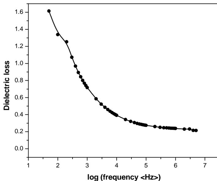
Fig 7 Plot of dielectric loss versus log frequency
