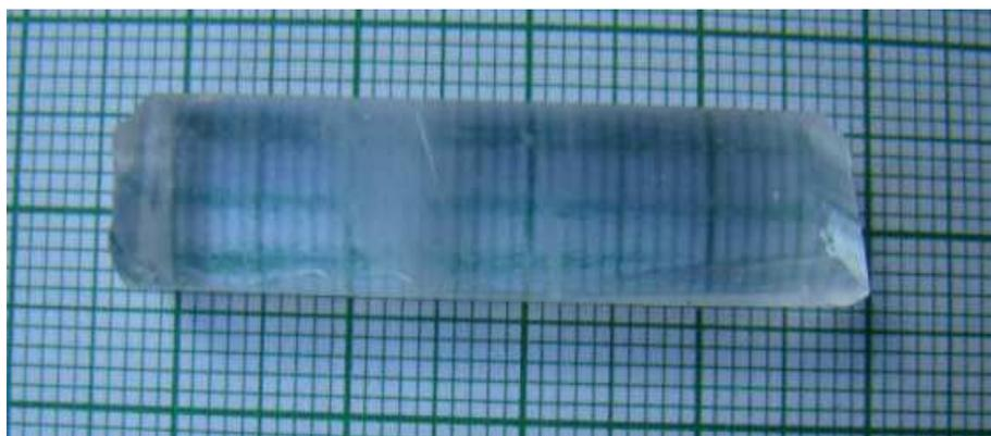
**Fig.1. LAIA crystal grown by SR method**
